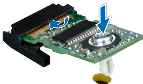
Figure 126. Installing the TPM
