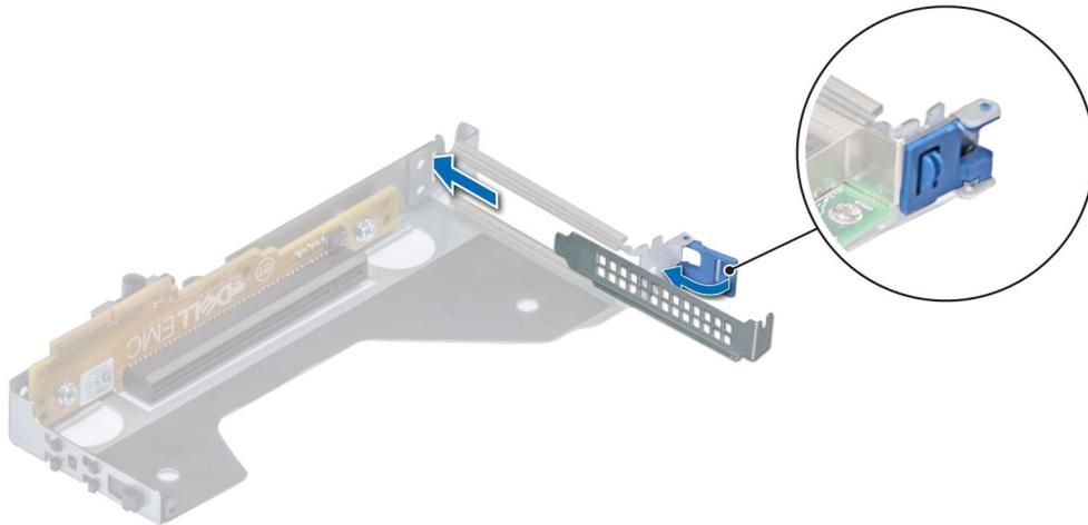
**Figure 81. Installing a filler bracket for riser 2**
