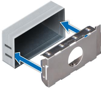
Figure 121. Installing a power supply unit blank
