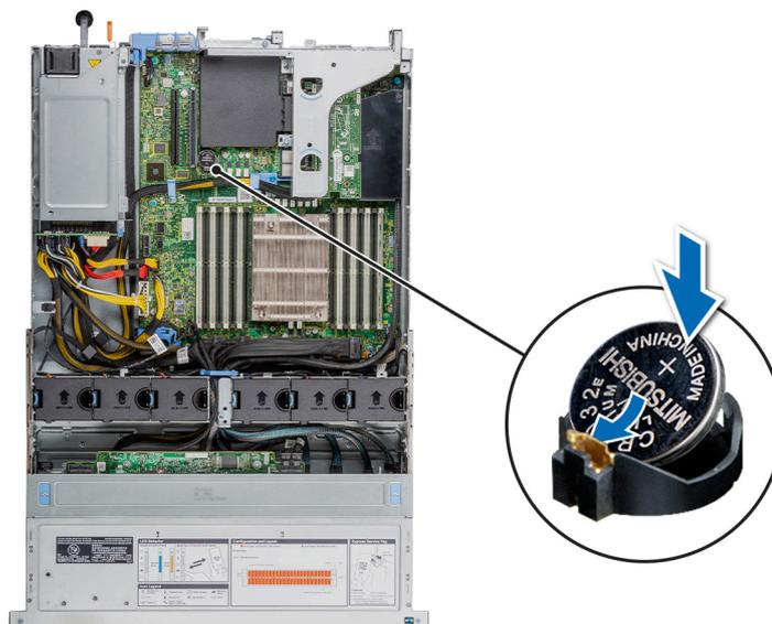
**Figure 111. Installing the system battery**
