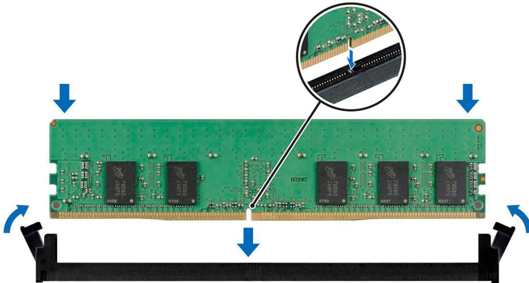
**Figure 56. Installing a memory module**
