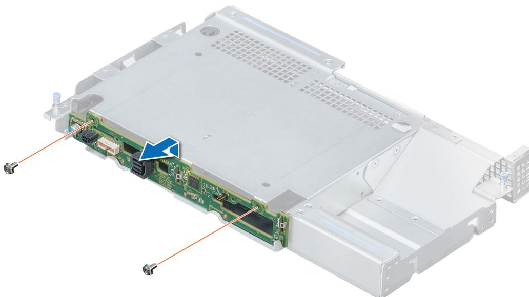
**Figure 51. Removing the rear drive backplane**
