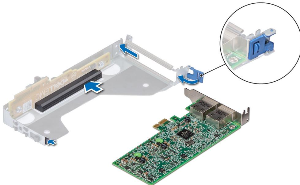
Figure 87. Installing the expansion card into a riser 2
