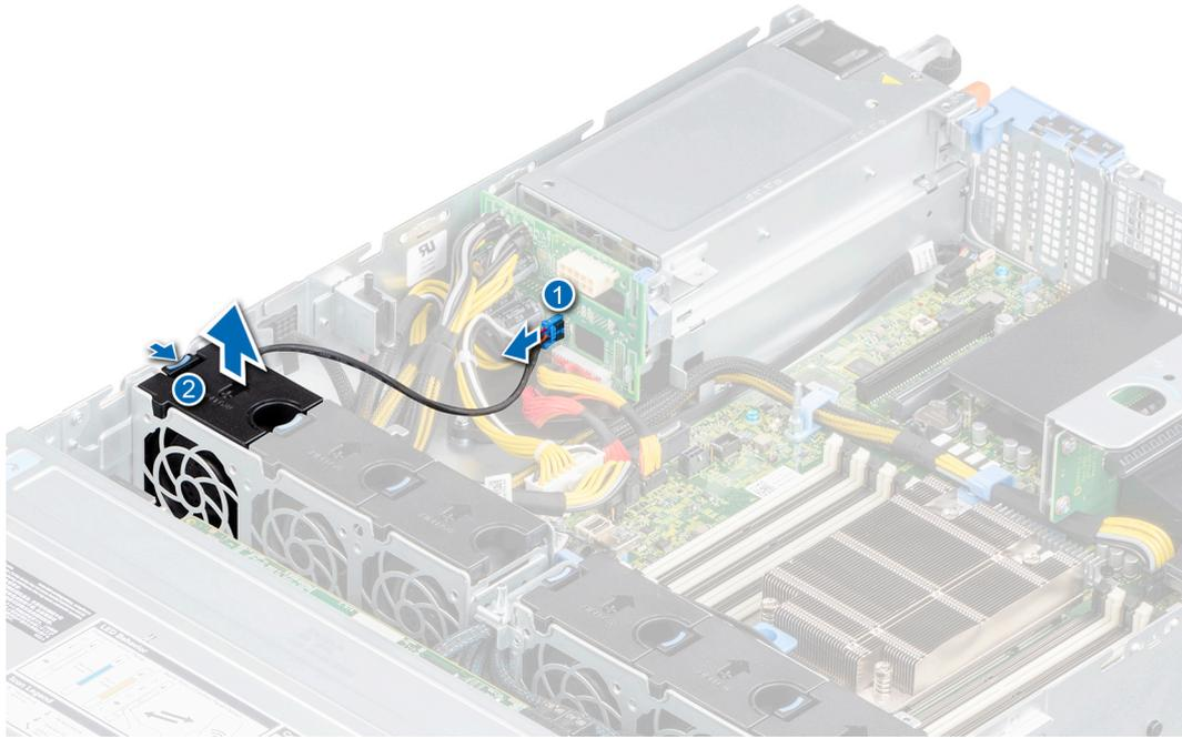
**Figure 28. Disconnecting fan 1 cable from PIB**
