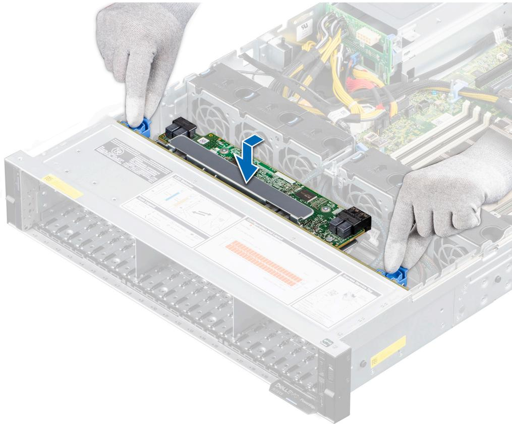
**Figure 50. Installing the drive backplane**
