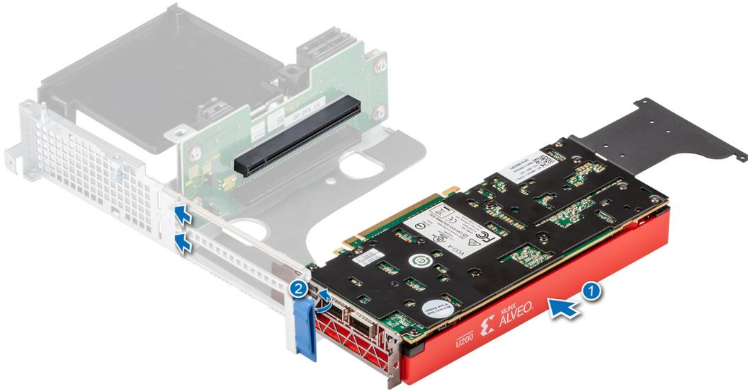
**Figure 91. Installing the accelerator card into riser 1B**
