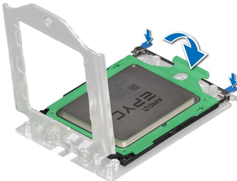
**Figure 62. Closing the rail frame**
