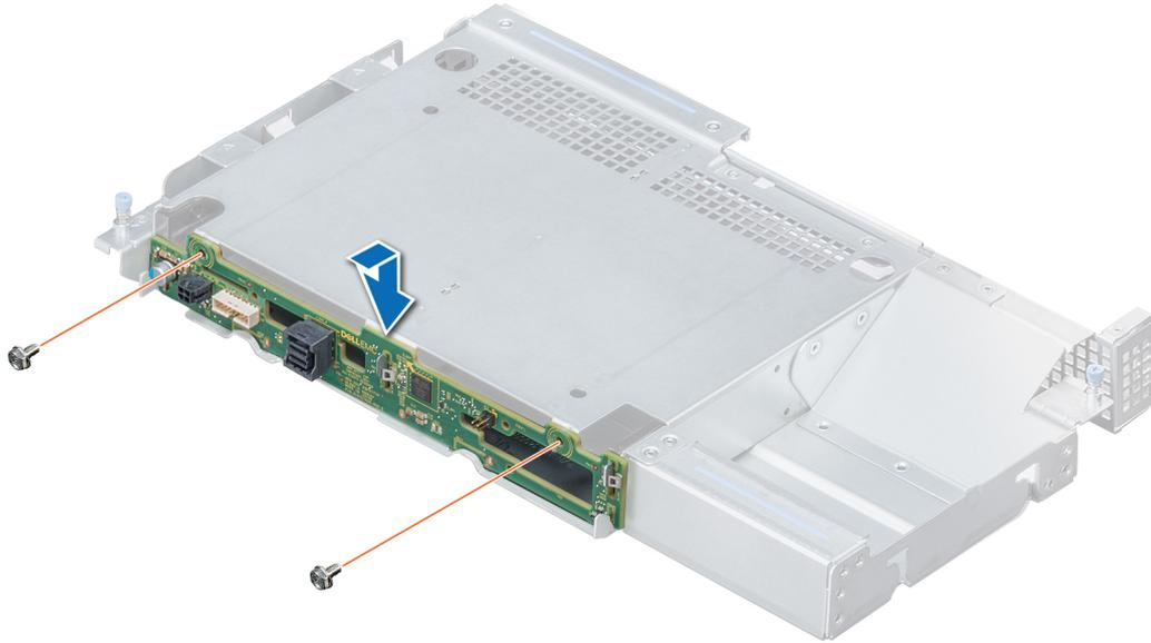
**Figure 52. Installing the rear drive backplane**
