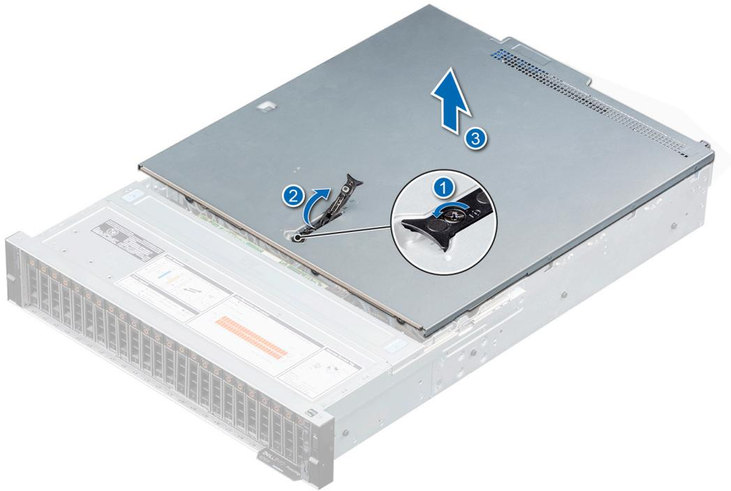
**Figure 19. Removing the system cover**
