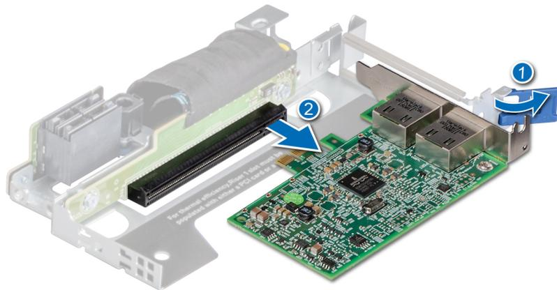
Figure 77. Removing the expansion card from riser 1A
