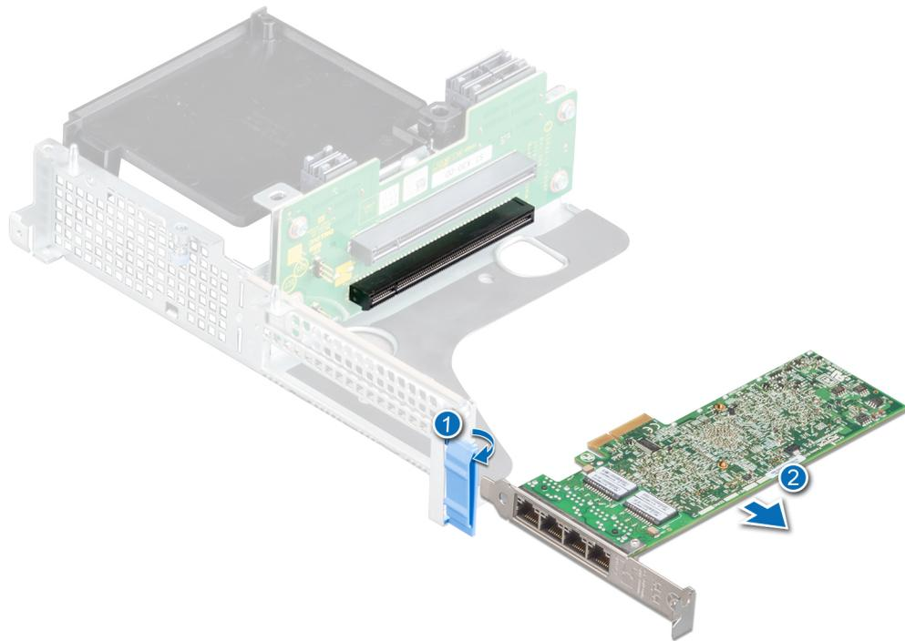
Figure 76. Removing the expansion card from riser 1B
