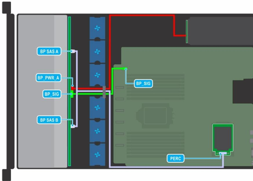
Figure 40. Cable routing - 8 x 3.5 inch drive backplane with mini PERC card
