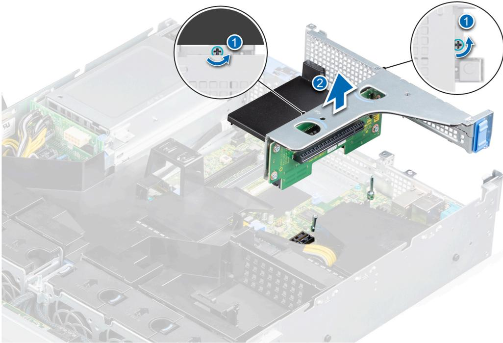
**Figure 68. Removing the riser 1B**
