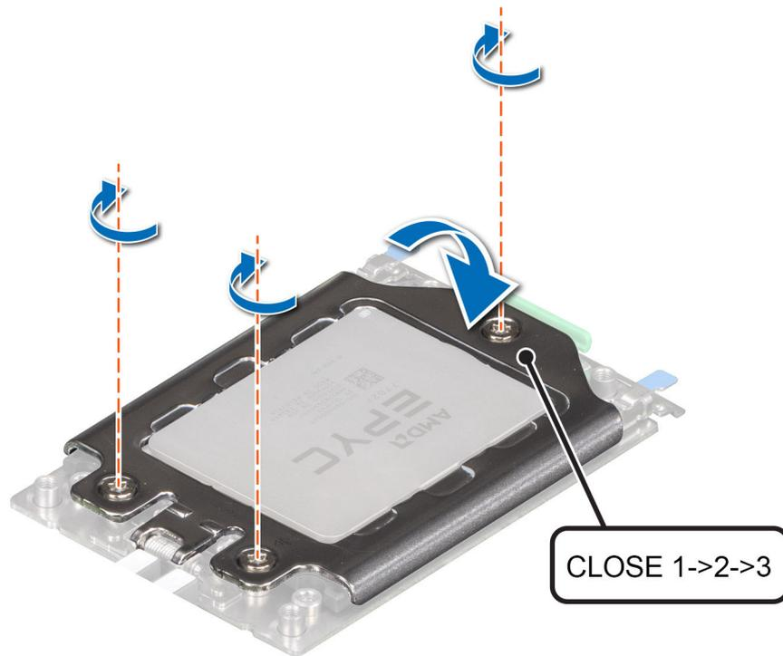
Figure 63. Securing the force plate
