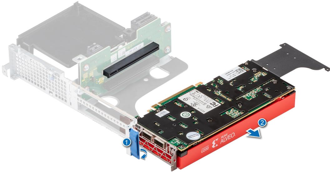
**Figure 90. Removing the accelerator card from riser 1B**
