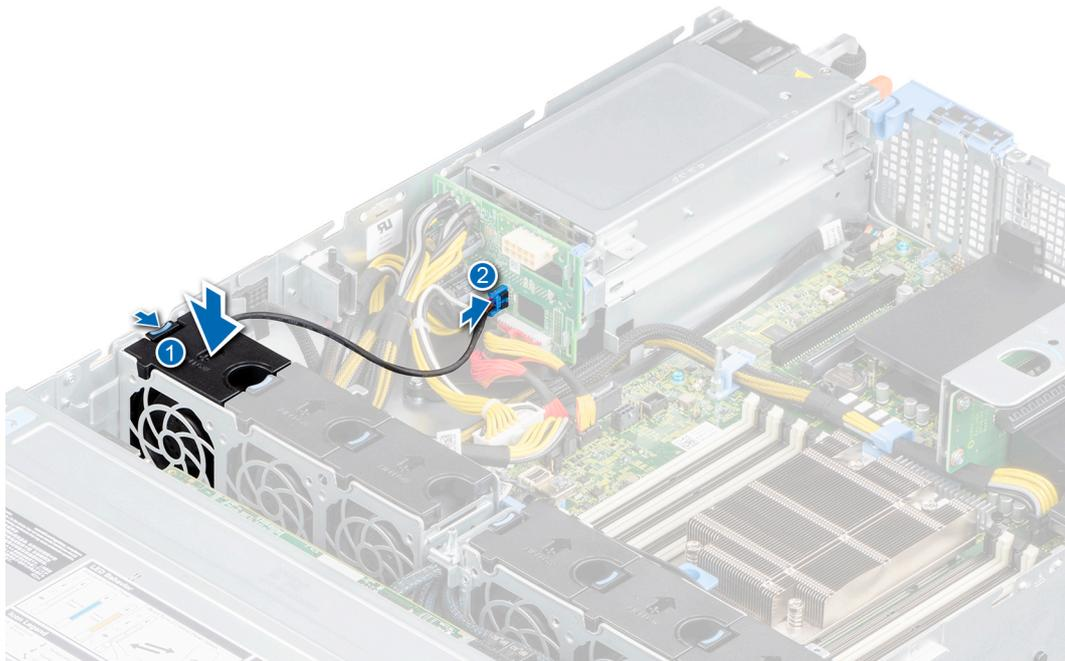
**Figure 30. Connecting fan 1 cable to PIB**
