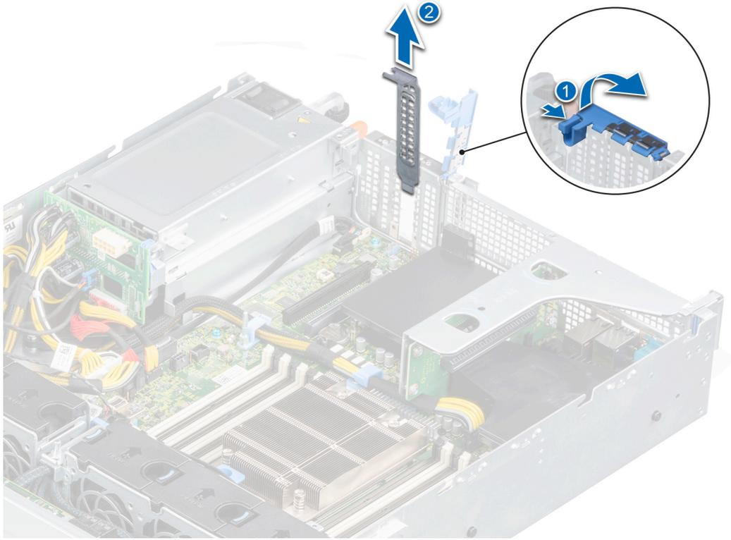
**Figure 74. Removing the filler bracket**
