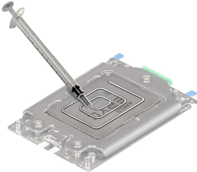
**Figure 64. Applying thermal grease on the processor**
