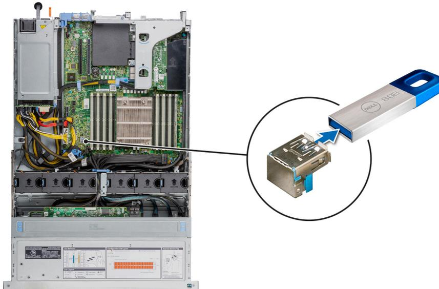
**Figure 112. Removing the internal USB memory key**
