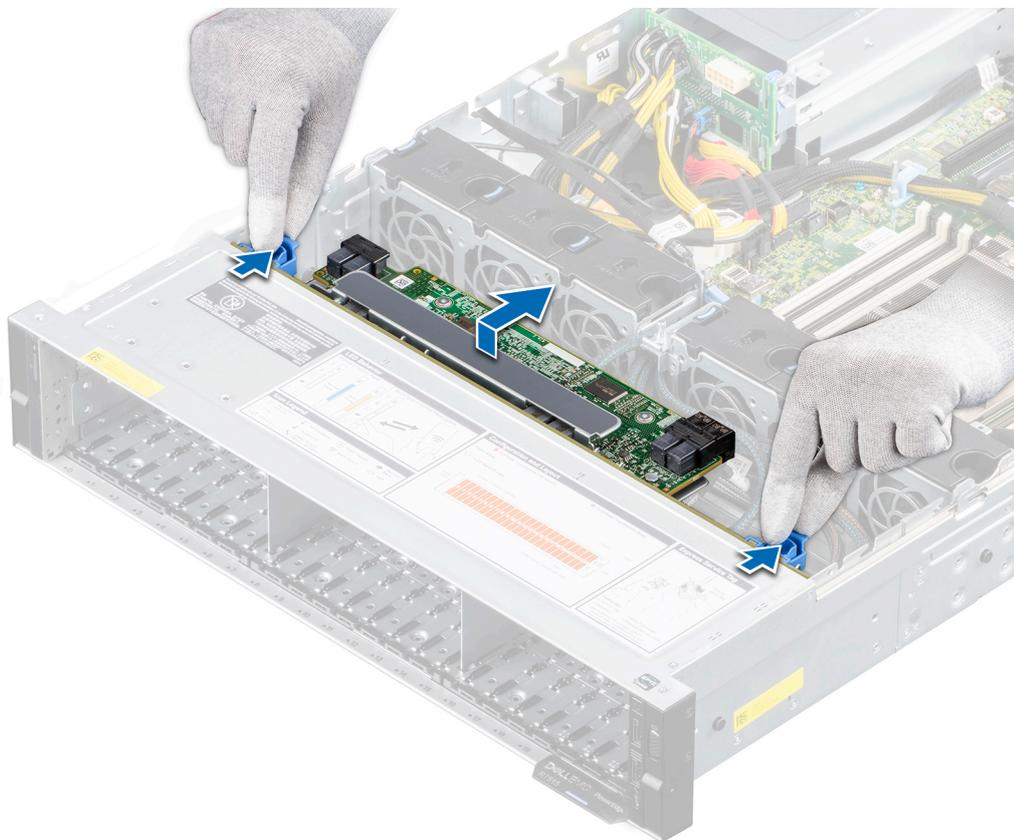
**Figure 49. Removing the drive backplane**
