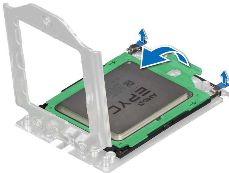
**Figure 59. Lifting the rail frame**
