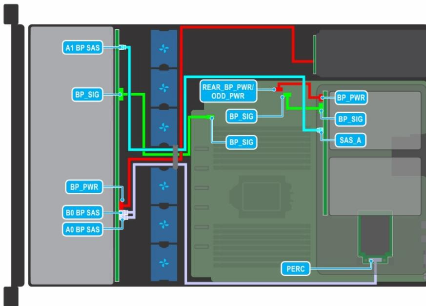
Figure 41. Cable routing - 12 x 3.5 inch drive backplane with 2 x 3.5 inch rear drive backplane
