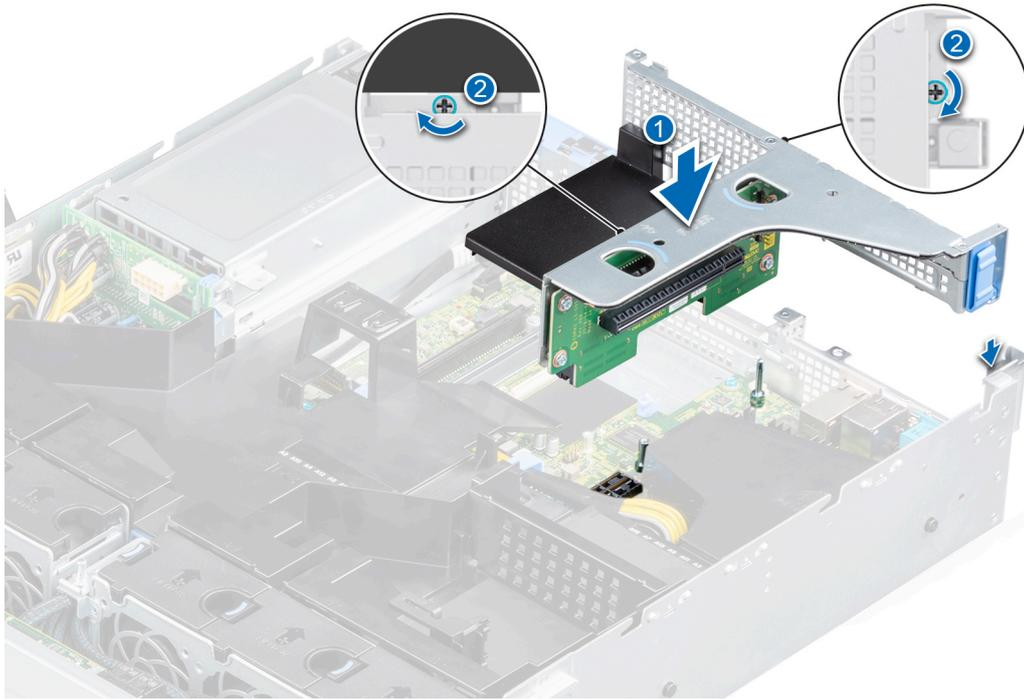
**Figure 71. Installing the riser 1B**
