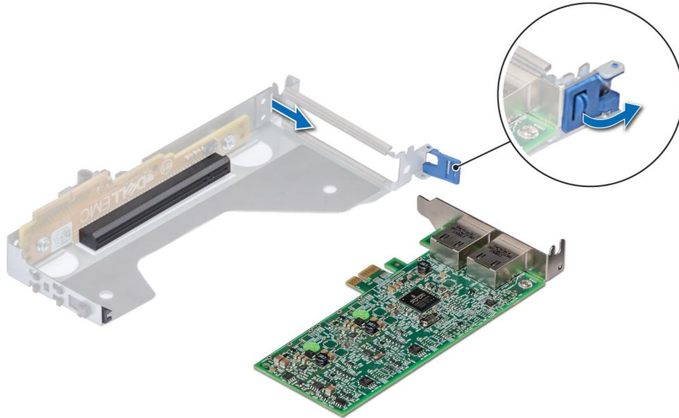
**Figure 78. Removing the expansion card from riser 2**
