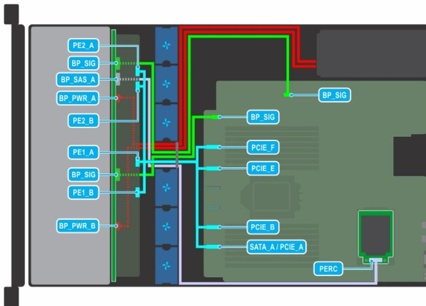
Figure 43. Cable routing - 24 x 2.5 inch NVMe drive backplane
