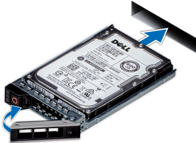
**Figure 36. Installing the drive carrier**
