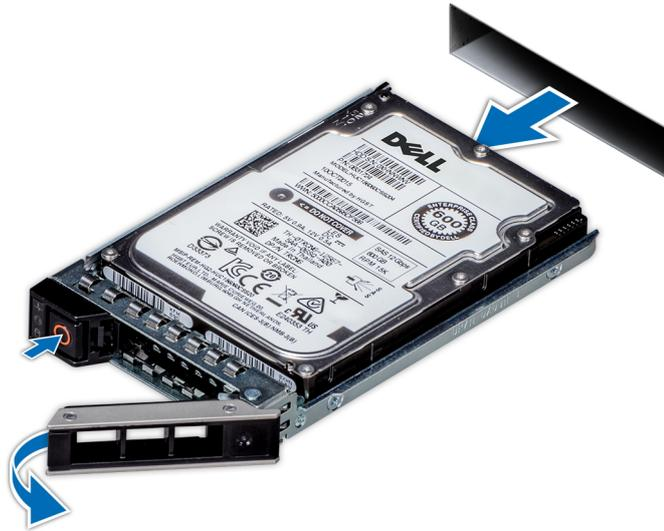
Figure 35. Removing the drive carrier
