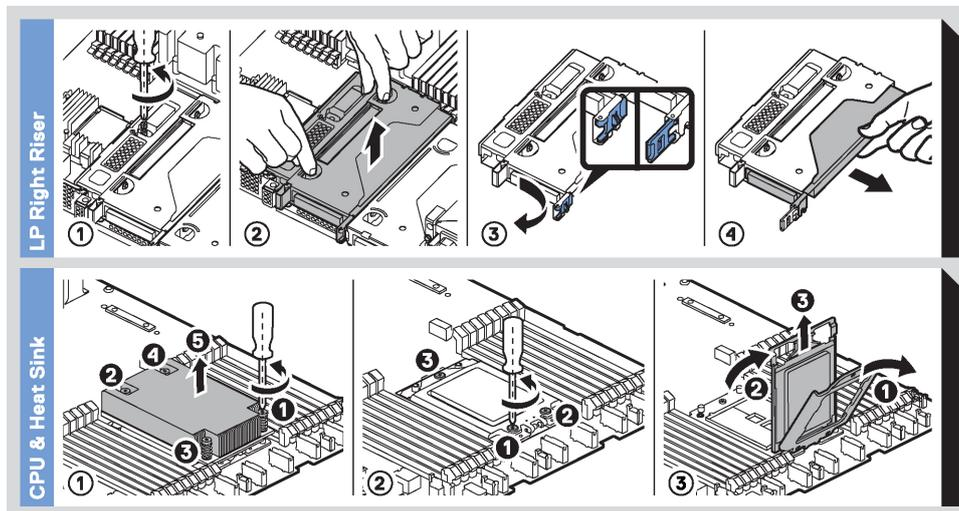
Figure 14. CPU and heat sink and LP right riser
