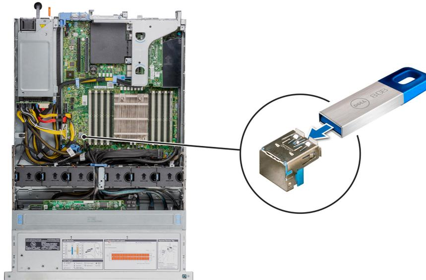
**Figure 113. Installing the internal USB memory key**
