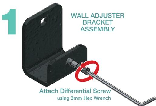
2. Attach two (2) Wall Adjuster Brackets to the back side using a 3mm hex wrench.
