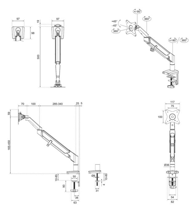
Neomounts Measuring unit: mm
