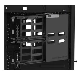
**Tool-less HDD Cage**
