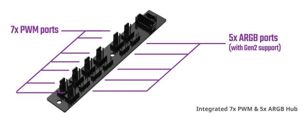
This chassis features a fully integrated PWM/ARGB Hub that allows for effortless cable management and control over multiple fans and ARGB devices. The Hub is fully compatible with ARGB Gen2 devices, allowing users to customize fan speeds and ARGB effects in depth according to their system needs or personal preference.
