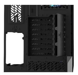
Tool-less Vertical GPU Mounting (Patent Pending)
