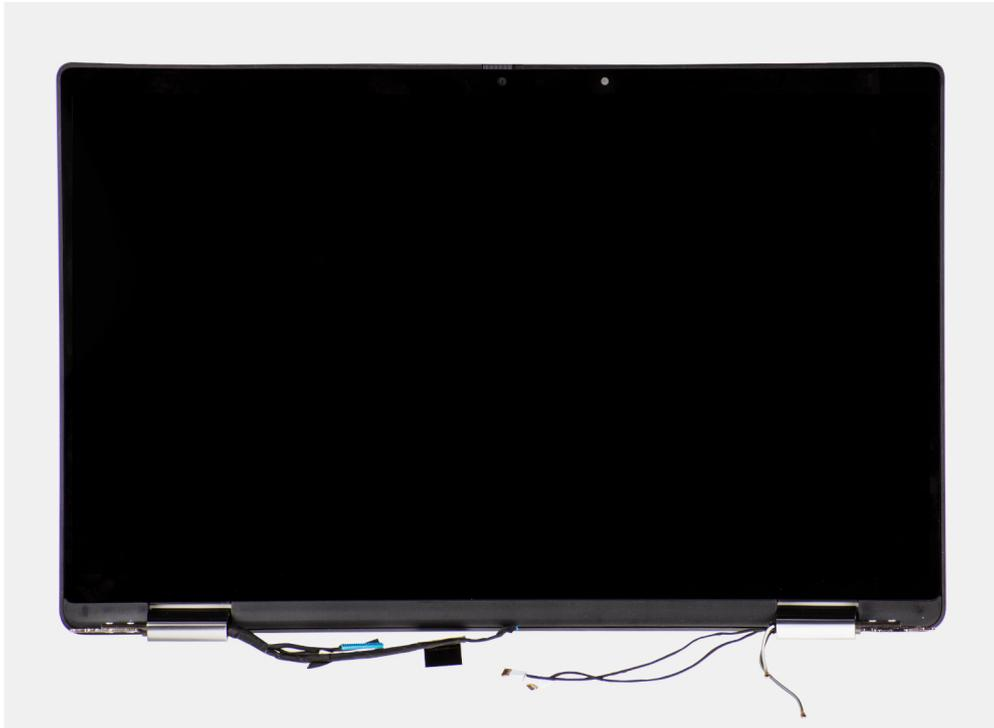
**Figure 1. Display assembly with antennae cables**
