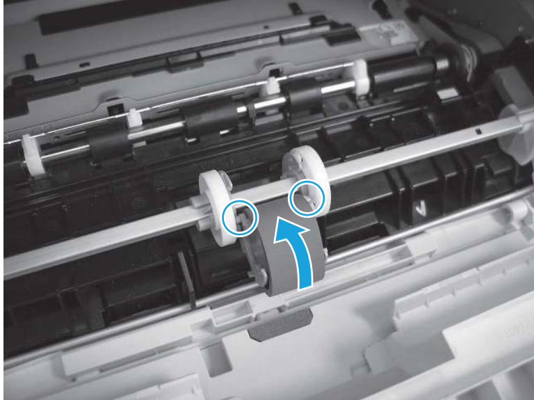
Figure 9-13 Install the roller
