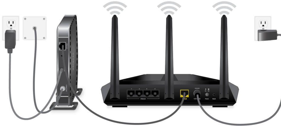
Figure 6. Cable your router
