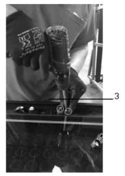
The lock is removed by unscrewing the 2 screws shown above.
