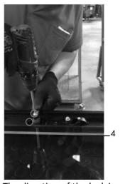
The direction of the lock is changed. Screws are assembled as shown.
