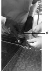
The removed hinge parts are attached to the other side of the door.
