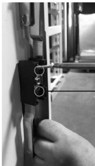
The direction of the lock is changed. Screws are assembled as shown.
