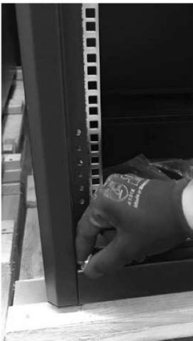
The pin located below is removed by turning
