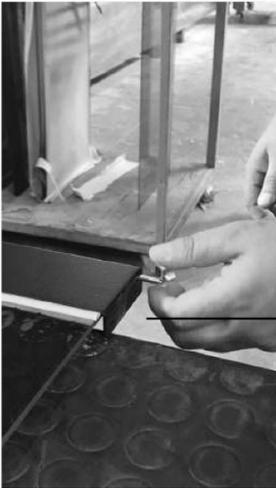
The hinge parts on the upper part of the door are removed.
