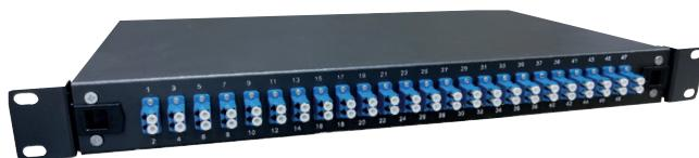
19" Fibre patch panel for up to 24 SC Simplex or LC Duplex adapters. The panel back side features 4 Ø20 mm inlets suitable for PG screw connection and 2 rectangular inlets 80 x 34 mm with blank plates.
