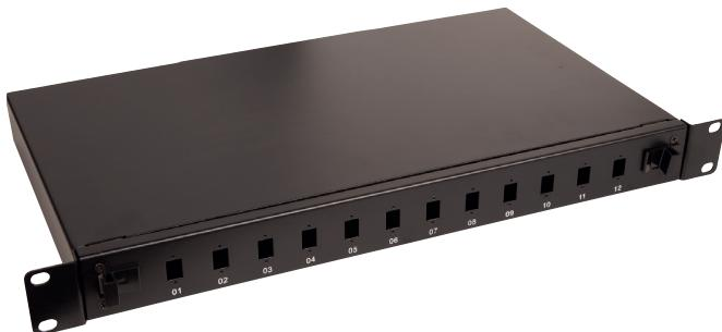
19" Fibre patch panel for up to 12 SC Simplex or LC Duplex adapters. The panel back side features 4 Ø20 mm inlets suitable for PG screw connection and 2 rectangular inlets 80 x 34 mm with blank plates.
