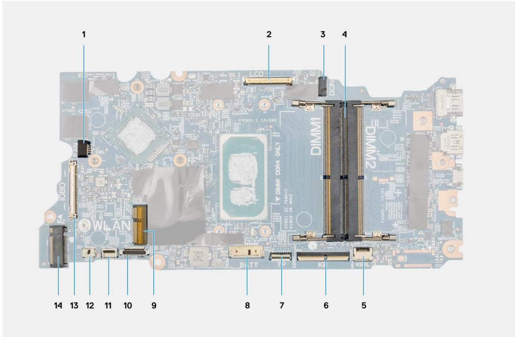
**Figure 2. System board connectors**
