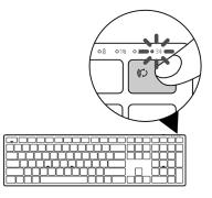
2 Press and hold the connection-mode button for 3 seconds to initiate pairing.
