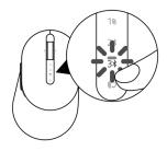
2 Press and hold the connection-mode button for 3 seconds to initiate pairing. The connection-mode light (3\*) blinks for 3 minutes, indicating your wireless mouse is in the pairing mode.
