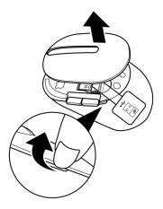
2 Remove the USB receiver from its compartment.
