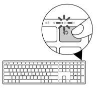
2 Press and hold the connection-mode button for 3 seconds to initiate pairing.
