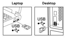
2 The connection-mode light (1) on the wireless mouse turns on to indicate the Dell Universal pairing, and then turns off.
