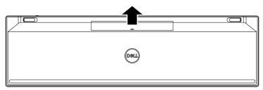
2 Install the AAA batteries into the battery compartment.
