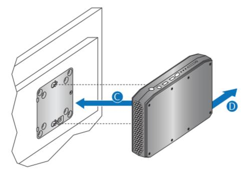
3. Place and slide the Intel NUC onto the VESA mount bracket (C and D)
