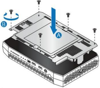
2. Place the top lid on top of the metal plate (C) and secure the screws with the screwdriver (D).
