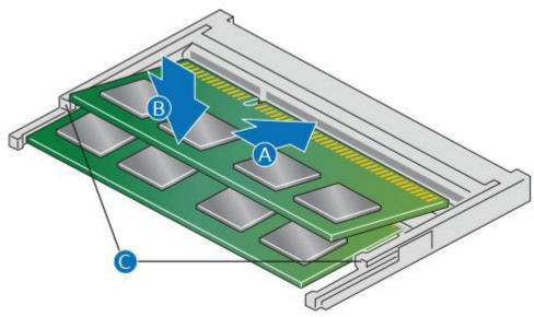
6. When the module is inserted, push down on the outer edge of module until the retaining clips snap into place (B). Make sure the clips are firmly in place (C).
