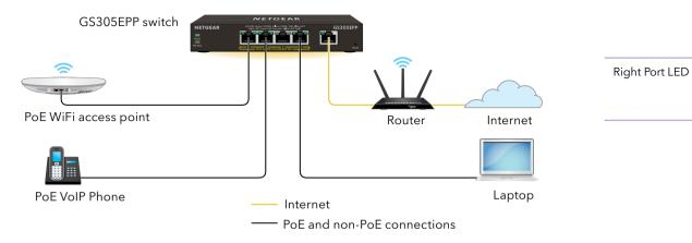
Note: We recommend that you use a Category 5e (Cat 5e) cable or higher-rated cable for Gigabit Ethernet connections.
