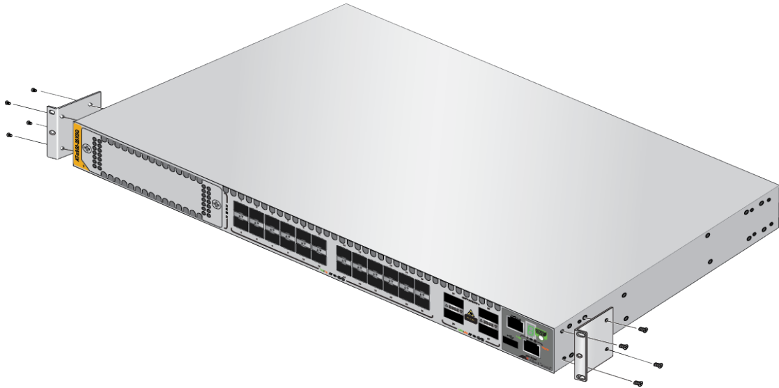
Figure 85. Attaching the Equipment Rack Brackets
