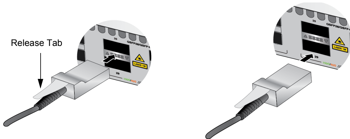
Figure 134. Attaching QSFP+ Cables
