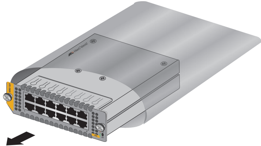
Figure 73. Removing the Ethernet Line Card from the Anti-static Bag
