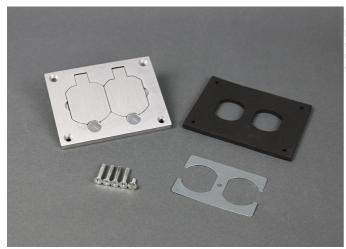
Brushed aluminum duplex cover plate, for OmniBox® and Modulink™ Series floor boxes. Cover plate is 3.290 inch x 4.310 inch (83.6mm x 109.5mm). Flip lids can also be used with 106 type frames for communications. NOTE: Brass covers and flanges are not interchangeable with aluminum or nonmetallic covers and flanges. Nonmetallic covers are interchangeable with aluminum flanges.
