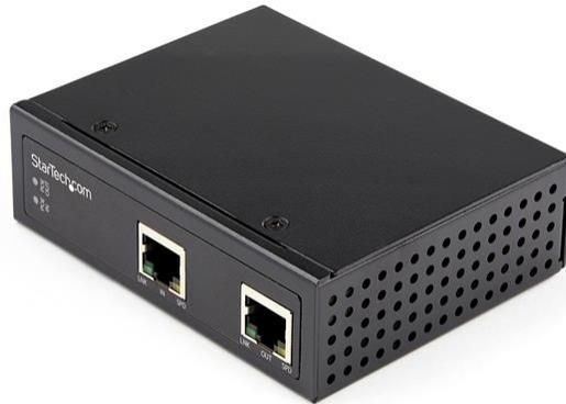
Extends the reach of PoE links up to 328' (100 m) to power powered devices (PD) over long distances; up to 4 extenders can be cascaded to extend the range of a PoE source (PSE) device up to an additional 400m, for a total range of 500m from the original PSE source to the target device.
