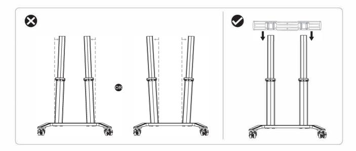
If the columns are not properly aligned, the mounting plate may fail to attach to the columns. Follow the steps below to re-assemble the columns.
