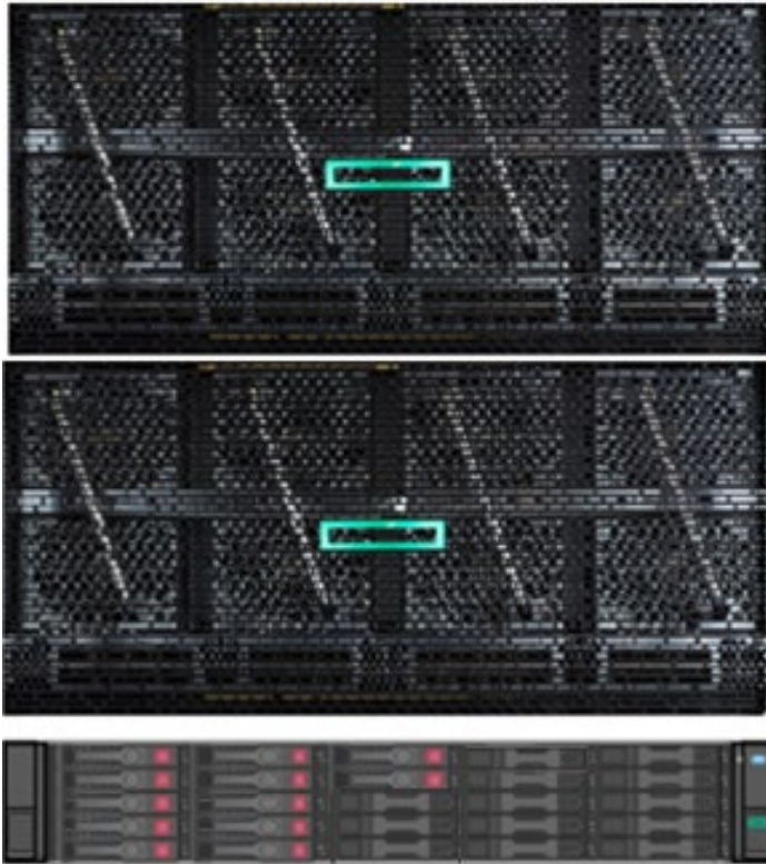
FIGURE 9. HPE Superdome Flex 8s Base Chassis Server with external D3710 with 12 SSD
