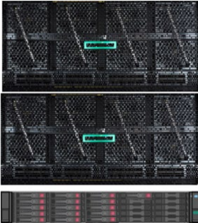
FIGURE 11. HPE Superdome Flex 8s Base Chassis Server with external D3710 with 16 SSD
