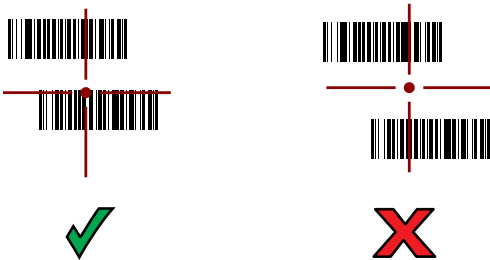
Figure 14 RS5100 Pick List Mode with Multiple Barcodes in Aiming Pattern
