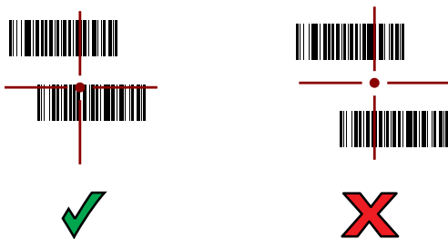
Figure 12 RS507/RS507X Pick List Mode with Multiple Barcodes in Aiming Pattern
