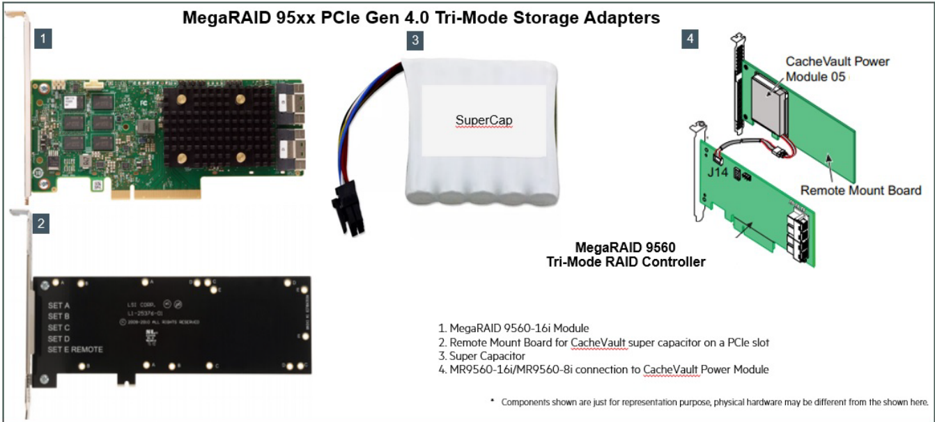
FIGURE 13. HPE Superdome-Flex 280 - MegaRAID 9560-16i and 9560-8i hardware components
