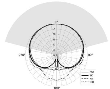
Figure 3b. Typical polar pattern (with full frequency response) of an Earthworks cardioid microphone
