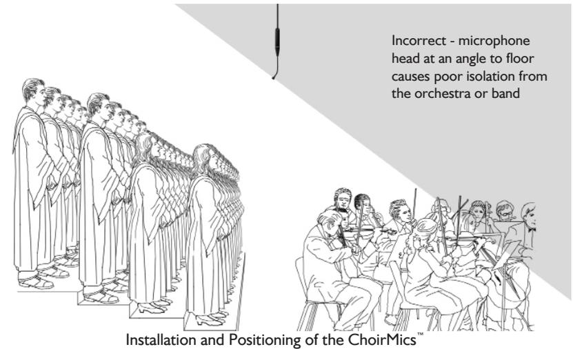
Figure 12. Improper Positioning of an Earthworks Cardioid Microphone with an Orchestra or Band behind the Microphone
