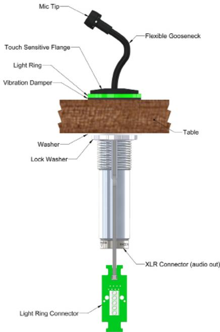
The light-ring emits a momentary digital pulse to the connector on the pc board to activate external control systems or equipment.
