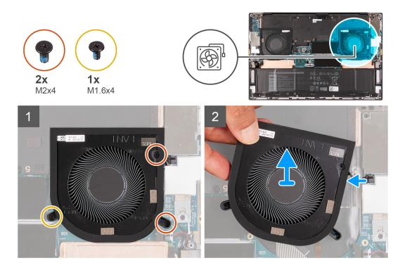
1. Remove the screw (M1.6x4) and the two screws (M2x4) that secure the right fan (FAN1) to the system board and palmrest and keyboard assembly.
