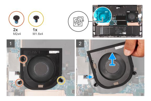
1. Remove the screw (M1.6x4) and the two screws (M2x4) that secure the left fan (FAN2) to the system board and palm-rest and keyboard assembly.
