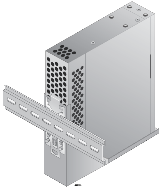
Figure 47. Verifying the DIN Rail Installation
