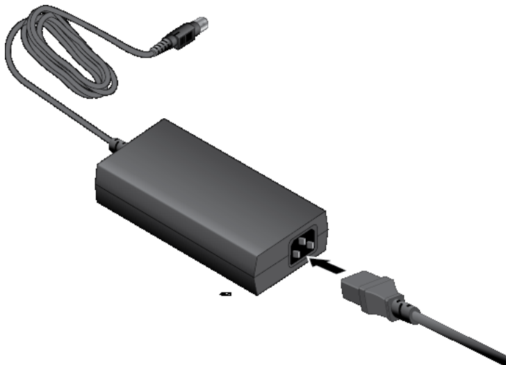
Figure 69. Connecting the Power Cord to the Power Adapter
