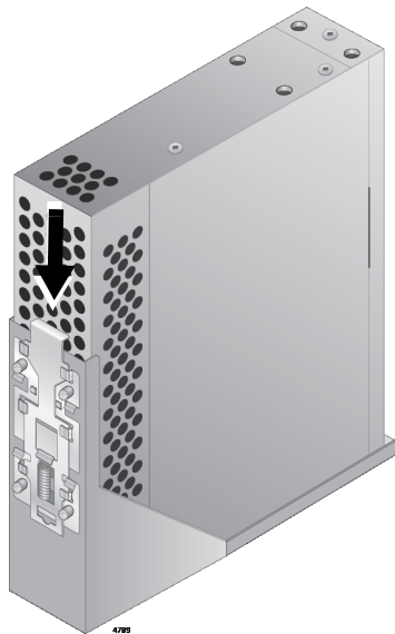
Figure 45. Pressing Down on the Spring-Loaded Lever
