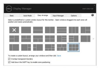
If you are using multiple displays in an array or matrix, **Easy Arrange** layout can be applied across to all the displays as one desktop. Select "**Span multiple displays**" to enable this feature. You need to align your displays properly to make it effective.
