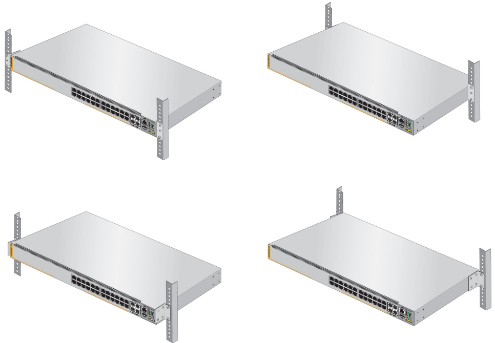
Figure 31. Switch Orientations in an Equipment Rack
