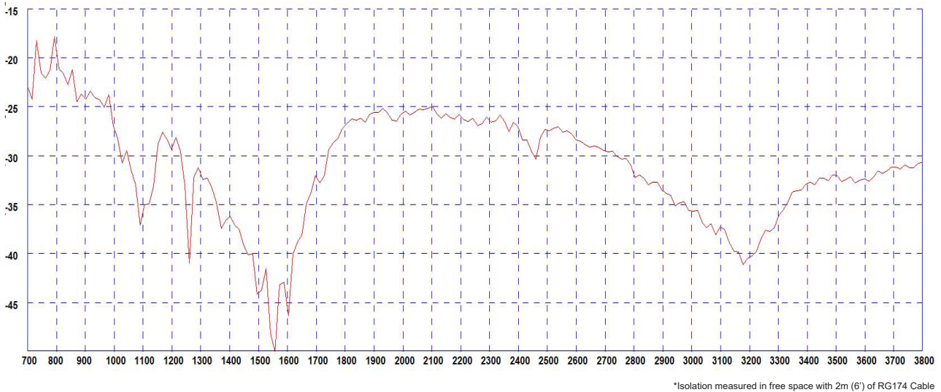
Typical Isolation Elements 1&2*
