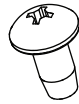
(4x) Thread Forming Screw (For Lever Lock™ Compatible Rackrail Bracket Installation) B
