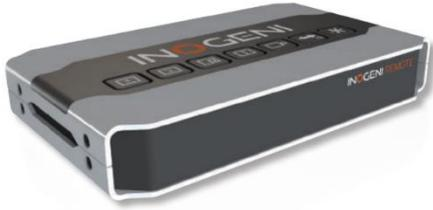
The INOGENI Remote needs to be connected to the terminal block port in order to operate. Apply wiring accordingly. This remote is sending serial commands to the CAM device. Make sure to set the DIP SW6 for CAM100 and CAM300 devices in order to apply power to the remote before going further. See “DIP SWITCHES” section of this document for more details. Check the user manual of the INOGENI REMOTE for more details.
