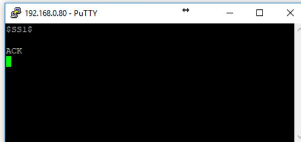
You can use the commands by sending HTTP or TCP requests. For example, you can send an HTTP request by sending it using any browser, for example, to 192.168.0.80:50000/COMMAND. If the command is recognized, you will receive the ACK string.
