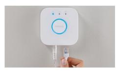
The Hue Bridge\*, the heart of your smart lighting system, connects your Hue White and colour ambience smart lights to your app and the sync box, allowing you to customise and save your light settings when syncing. \*The sync box is only compatible with the square-shaped Hue Bridge V2.
