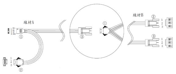
[Step 2] Connect Cable B's connectors ② and ③ to addressable RGB devices
