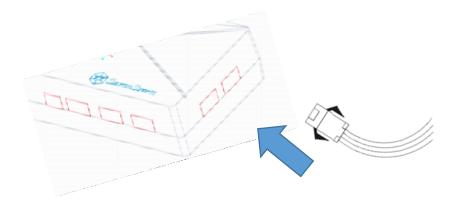
[Step 2] Connect Cable A's connector 3 to an addressable RGB device
