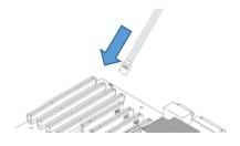
**1.2 Signal source – addressable RGB controller / box / hub:** Connect Cable A's connector **2** to controller's pin header (e.g. SilverStone LSB02, CPL02)
