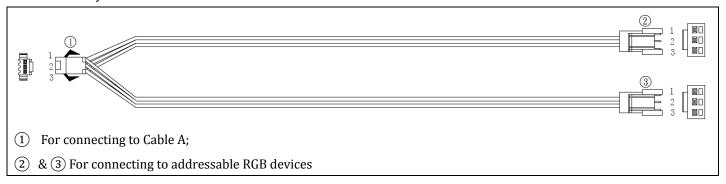
[Step 1] Connect Cable A's connector 3 to Cable B's connector ①
