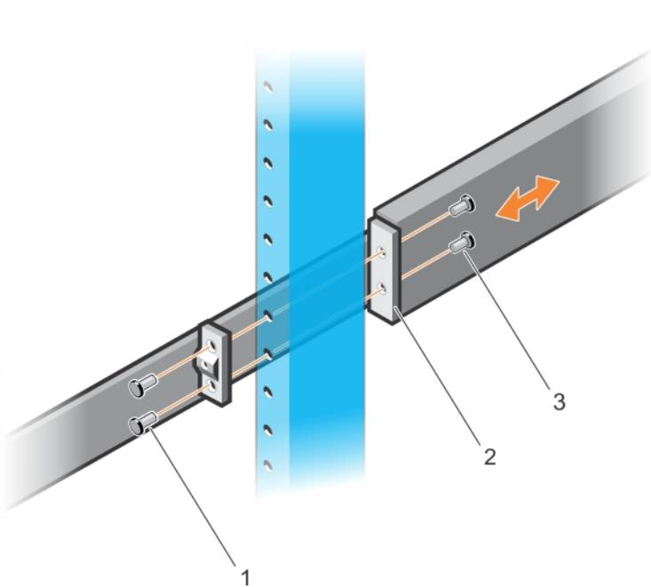
**Figure 14. Two-post center-mount installation**
