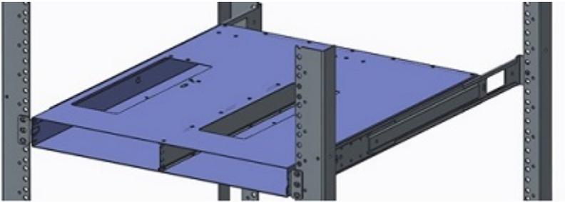
**Figure 6. Secure the dual-tray in the four-post rack**
