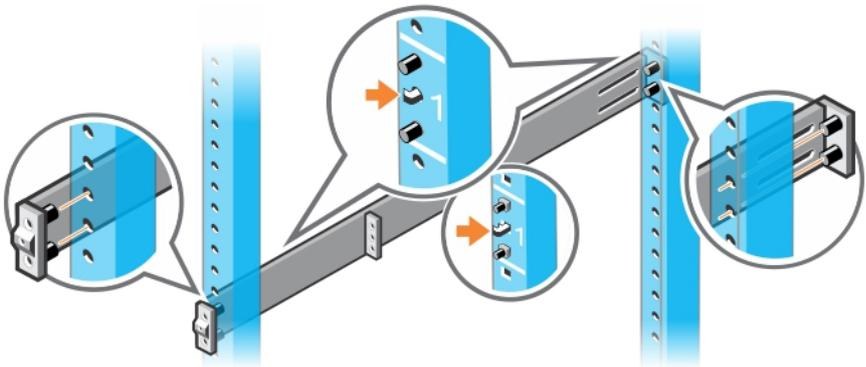
**Figure 12. 1U tool-less installation**
