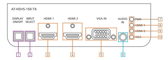
1. DISPLAY ON/OFF button: Sends RS-232 trigger command when used with a compatible receiver (e.g. AT-UHD-CLSO-824 - see CLSO manual for instructions)
