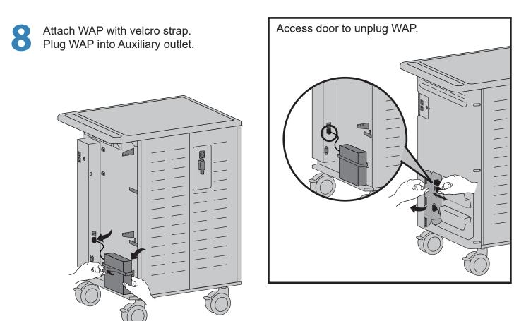
Attach side cover and plug power cable back into cart. NOTE: Route WAP Ethernet cable through side cover access door.
