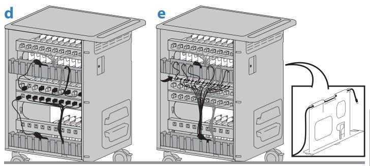
g. Plug in the power cables for the bottom shelf. Use the bottom row of outlets. Store the power cables in the bottom basket.
