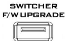
2. Insert the USB stick containing the latest firmware to the FW upgrade port.
