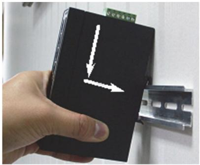
Install Industrial Equipment in DIN-Rail mount.
