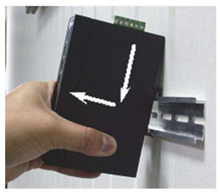
Remove Industrial Equipment in DIN-Rail mount.
