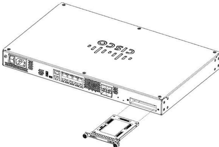
**Step 3** Tighten the thumb screws on both sides of the SSD bay.
