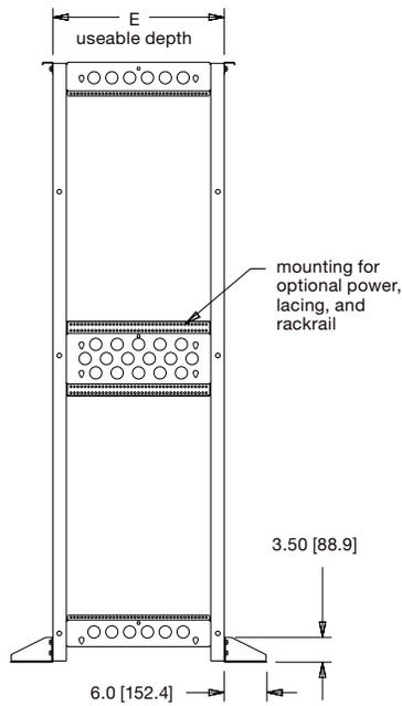
accepts 6", 9", and 12" cable ladder widths
