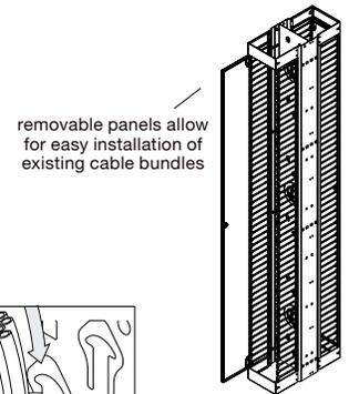
removable panels allow for easy installation of existing cable bundles
