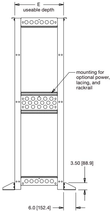
accepts 6", 9", and 12" cable ladder widths
