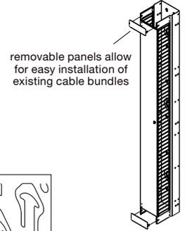
removable panels allow for easy installation of existing cable bundles
