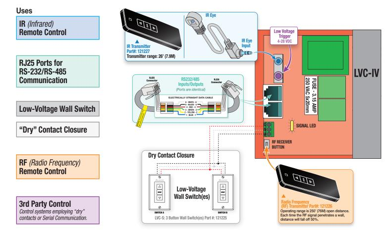
The 120V LVC-IV also used as a Single-Pole, Double-Throw dry closure to control equipment by the same means listed above.
