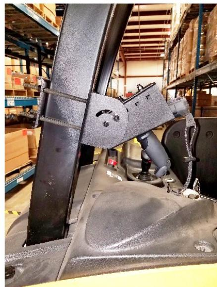
cap nuts to adjust width
