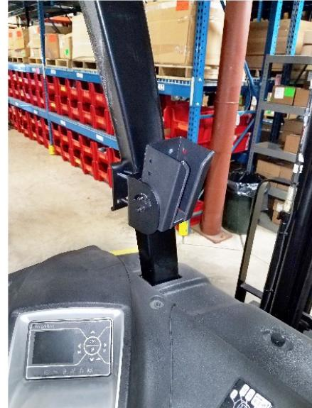
cap nuts to adjust width
