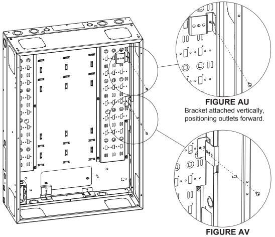
Bracket attached vertically, positioning outlets inside.
