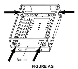
2. Install a vent guard into each of the 4 openings (from the outside into the enclosure) using a guard (A), (4x) 6-32 x 3/8" screws (M), and (4x) 6-32 flange nuts (B) in each location. (**FIGURE AH**)
