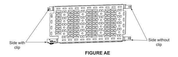
The Lever Lock backpan plate may be installed on the brackets at different depths. All 4 corners of the Lever Lock backpan plate must be inserted into the brackets at the same depth in order to function correctly.
