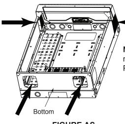
**NOTE**: If using a 4" AC fan option, be sure to bond it correctly. For more information, see "Connecting 4" AC Fan Options to Bonding Points" on page 18.
