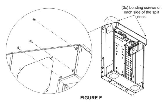
2. Carefully remove the split door and set it aside for reinstallation. (FIGURE G)
