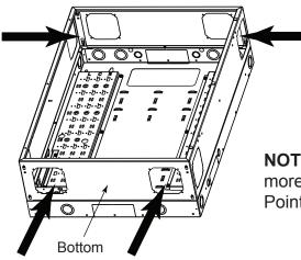
2. Install any 4" AC fan option (not provided, sold separately) into each of the 2 openings on the bottom of the rack using a fan, (4x) screws and (4x) nuts from the hardware provided with your fan. (FIGURE AL)
