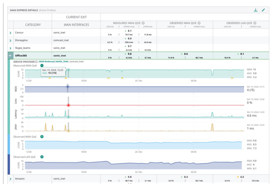
Figure 5. HPE Aruba Networking Central displaying measured versus observed QoE
