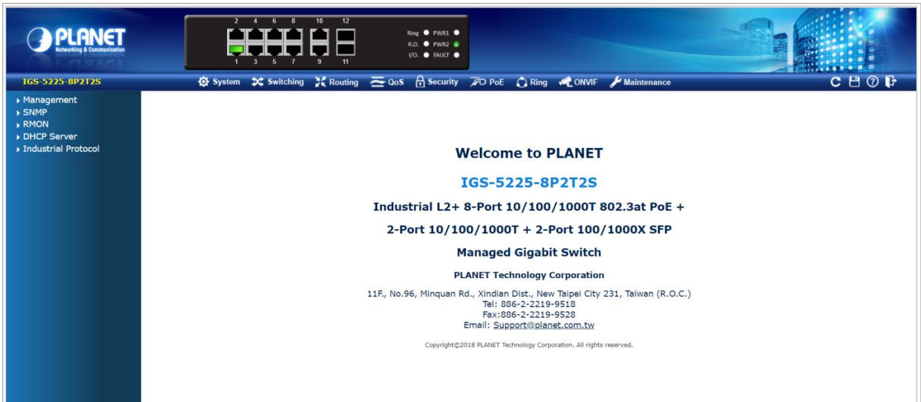
Figure 3-4: Web Main Screen of Industrial Managed Switch
