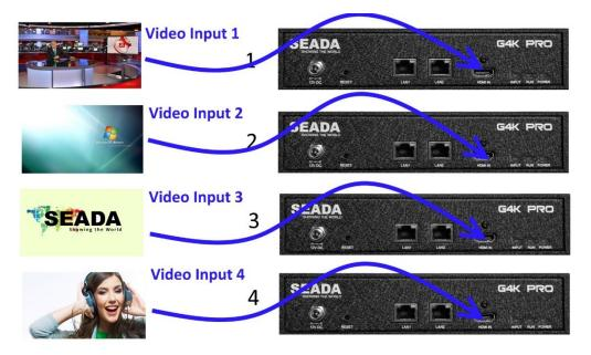
2. Inputs and Daisy Chain connections using HDMI cables.
