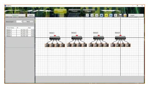
3) Click on the header of 1<sup>st</sup> device and drag the line to the 2<sup>nd</sup> device to open the 'Change Device Mode' dialog window to choose the Slave Mode (Daisy Chain mode) for the 2<sup>nd</sup> G4K Pro. And then 2<sup>nd</sup> to 3<sup>rd</sup> and 3<sup>rd</sup> to 4<sup>th</sup> unit.
