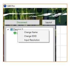
Users are able to change the input EDID of G4K Pro to match any shape of video wall layout. Go into 'Input' and then right click on the device needed EDID change and choose 'Change EDID' in drop down menu. The default path for EDID files are C:\G4KPro\Edid
