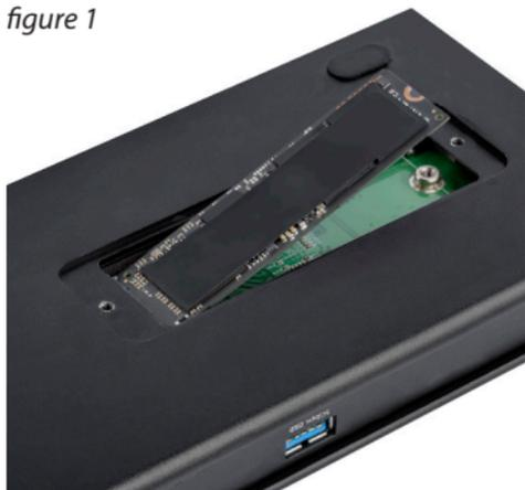
5. Gently press down on the M.2 drive until the notch on your M.2 Drive is aligned with the hole for the Holding Screw. Hold the drive in place.
