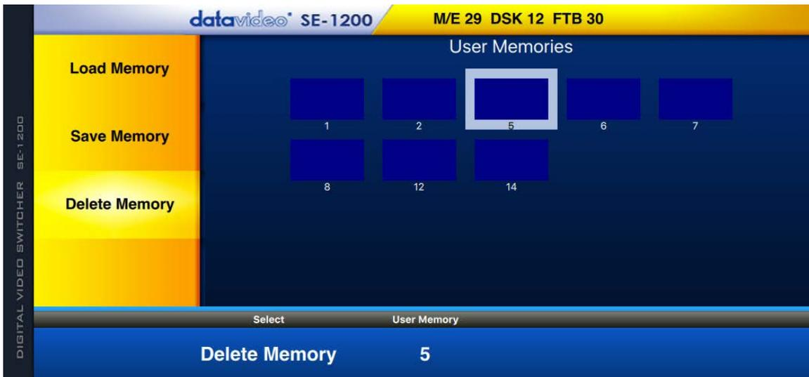
2. Select the User-defined setup to be deleted from User Memory slot matrix. **Be careful to select only the User memory slot to be deleted.**
