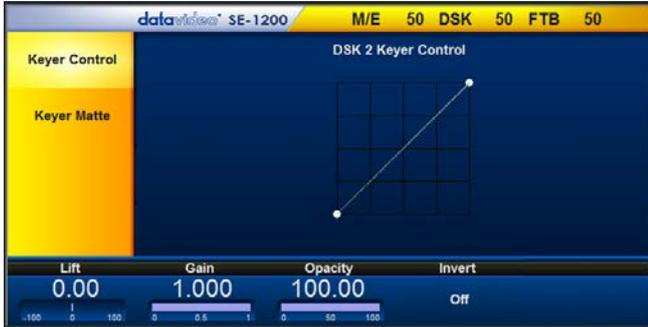
The options in the blue bar along the bottom of the Screen will allow you to calibrate for a white or black key using the **Lift, Gain, Opacity** and **Invert Functions**. The [Keyer Control section \(7.1.1\)](#) will explain the effects of **Lift, Gain, Opacity** and **Invert**.
