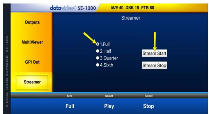
**Note:** The streamed SE-1200 MU multi view is video only, no audio is sent over this IP connection. If users choose Half rather than Full, it means that the streamed multiview video is transferred through IP network with less bandwidth.
