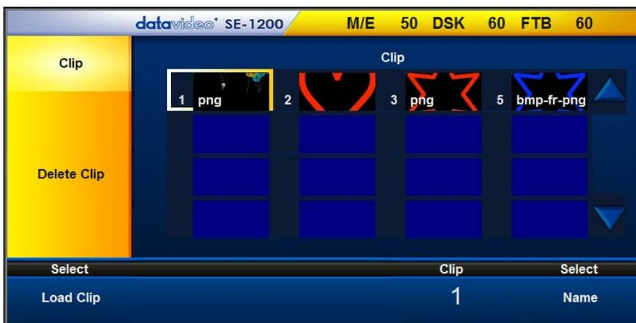
To load the clip, simply click on the **Clip** option and then select **“Load Clip”**. The clip is always loaded to input 6 so anything loaded to input 6 before will be replaced by the clip.
