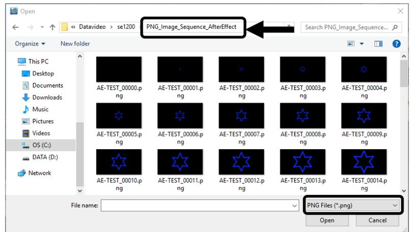
Click open to start the clip import. If your files are not the SE-1200 MU's .pic format, they will be automatically converted to .pic format by the SE-1200 MU PC Control APP first.
