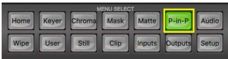
**Step 5:** Click the **P-in-P** button (backlit green) on the **MENU SELECT** panel to enter the Picture in Picture functions.
