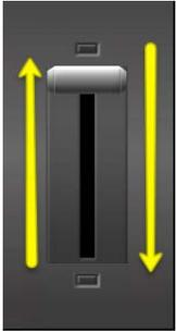
The timing of a **Clip** transition can also be manually decided when moving the **T-Bar** or completed over a set duration when using the **AUTO button**.
