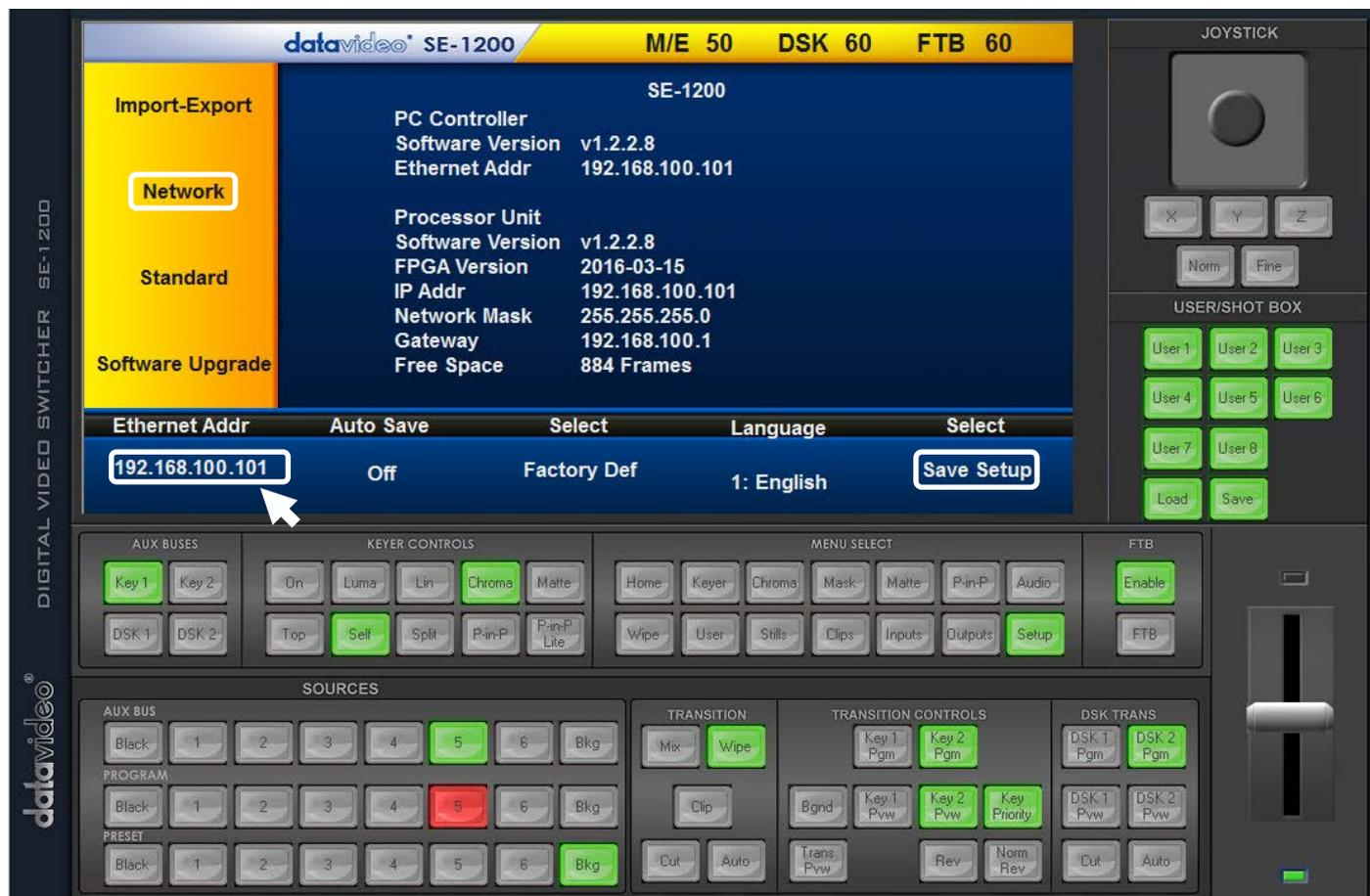
If the network settings are wrong then you may not be able to control the SE-1200 MU. Always keep a note of the last IP settings used and change these settings carefully to avoid problems.
