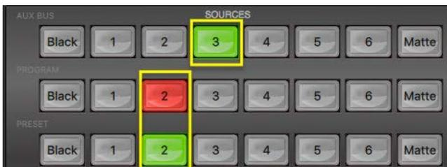
**Step 3:** The **Split button** is **backlit green**, select the **CG key source** on the **AUX BUS Row** (input 3).
