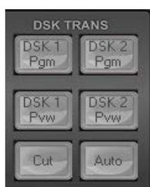
This panel is used to turn only the DownStream Keyers on or off. This can be done to show the chosen keyer in the Preview video output for configuration before live on-air use.
