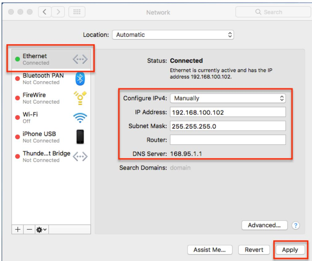
3. Please install the SE-1200 MU control software after setting the static IP of the iOS computer.
