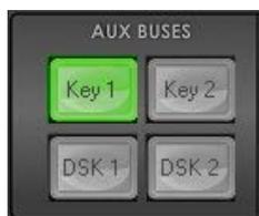
The SE-1200 MU has four dedicated keyers, **Key1**, **Key2**, **DSK1** and **DSK2**. All four keyers can be active simultaneously. **Key 1** and **Key2** can be set as Upstream or Downstream keyers.
