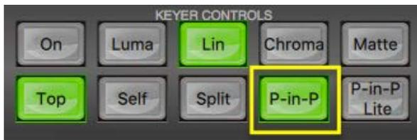
**Step 2:** Select the Key 2 effect by clicking the **P-in-P** button (backlit green) in the **Keyer Controls** panel.
