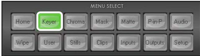
**Step 6:** To adjust the Luma key settings. Click the **Keyer button** in the **MENU SELECT panel** and the menu screen will appear as shown on the left here.
