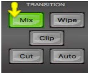
Pressing **Mix** will select a mix transition to use when moving from the current video source on the Program row to the selected next source on the Preset row.
