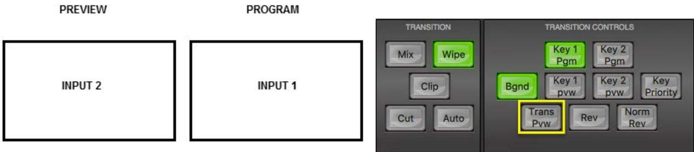
Using the **TRANSITION CONTROLS** panel click to select the **Trans Pvw** button (back lit green is ON). Next select and apply the transition or wipe that you would like to test on the Preview monitor.
