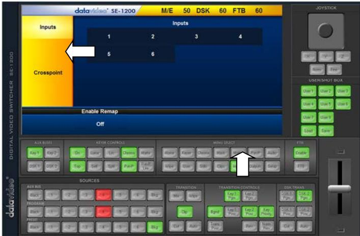
The physical input sources can be swapped around within the SE-1200 MU by using the **cross point** section of the **Inputs** menu.
