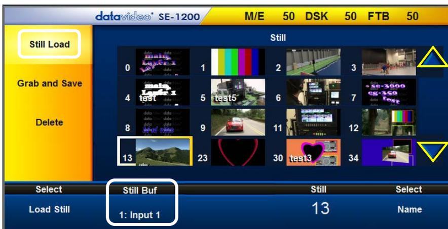
4. Change the **Still Buf option** in the lower row of options **to match the desired bus channel** that you wish to use to display the still image. In our example we have chosen **Input 1**.
