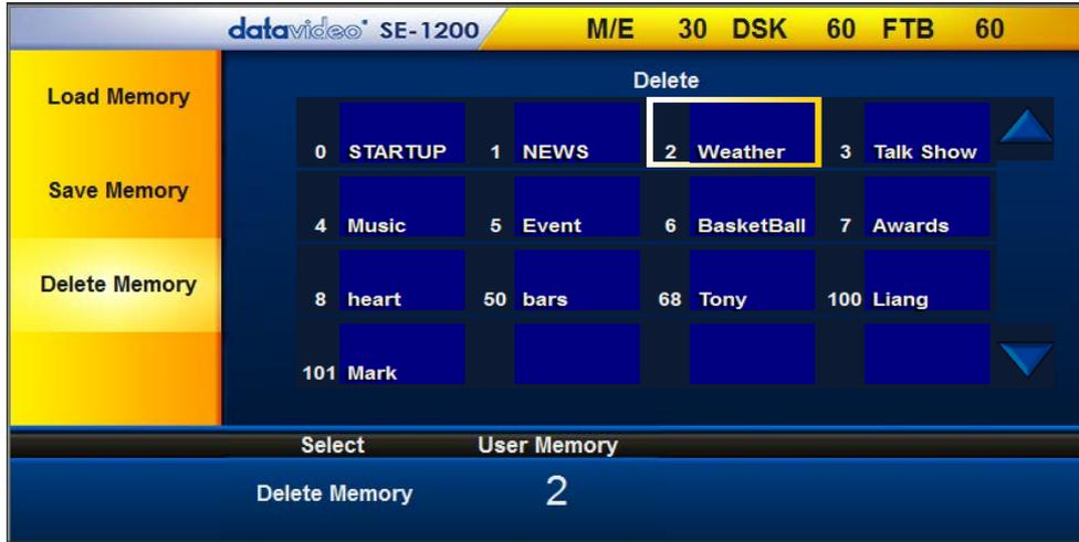
2. Select the User-defined setup to be deleted from User Memory slot matrix. **Be careful to select only the User memory slot to be deleted.**
