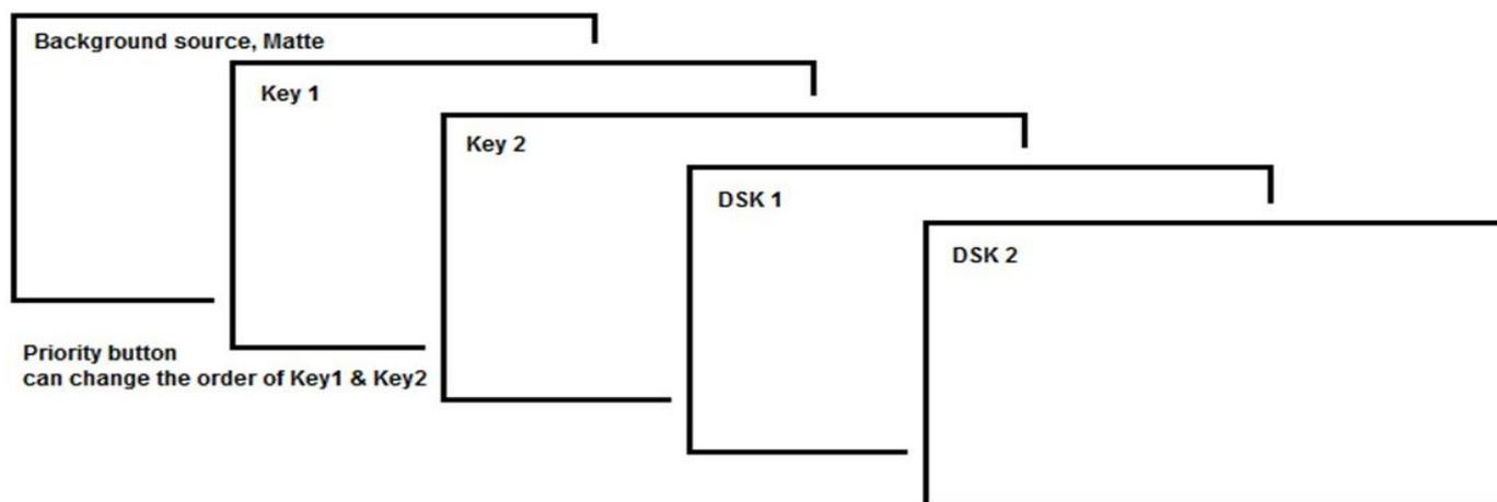
The **background video layer** is used for transitioning between Preview and Program sources. This layer also includes any selected wipe transitions. This layer can be hidden or partly hidden by the PiP, Keyer or DSK video layers in front of it.
