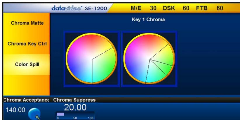
The **Color Spill** parameters and values are shown along the bottom of the display below. These settings are used to control/remove any unwanted Chroma or colour Spill from the background onto the foreground subject. There are two sectors drawn on the **Chroma** palette, one represents the wider **Chroma Acceptance** range and the narrower **Chroma Suppress** range.
