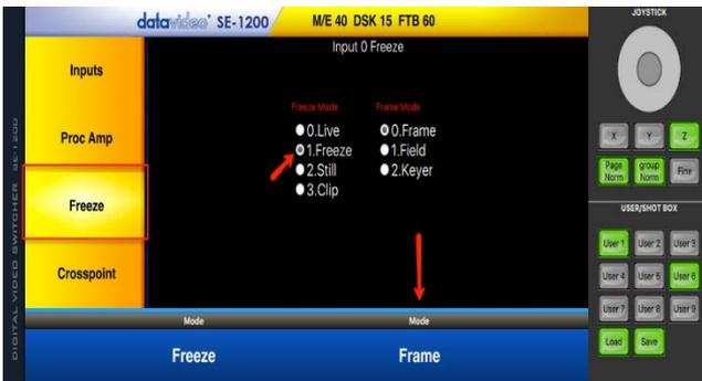
3. The Freeze parameters will then be displayed along the bottom row of the screen.
