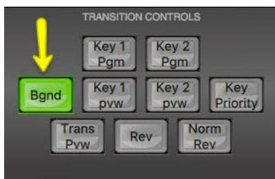
In order to enable clip transition between two video sources first ensure the Background Transition or **Bgnd** button is ON / backlit green in the **transition controls** area of the user interface.
