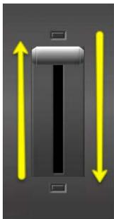
The timing of a **Mix** transition can also be manually decided when moving the **T-Bar** or completed over a set duration when using the **AUTO** button.
