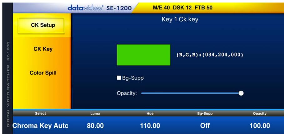
This matte sets the center of colour range that will be used for keying. The **Chroma Matte** parameters and the values are shown along the bottom of the display below.
