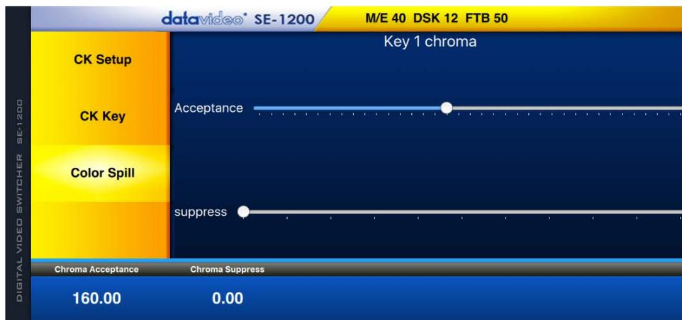
The **Color Spill** parameters and values are shown along the bottom of the display below. These settings are used to control/remove any unwanted Chroma or colour Spill from the background onto the foreground subject. There are two kinds of ranges in the **Color Spill** option including the **Chroma Acceptance** range and the **Chroma Suppress** range. Users can adjust their needed value by using the **Acceptance** and the **Suppress** sliders.
