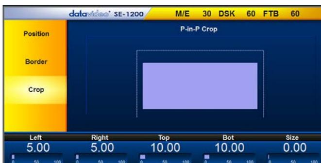
The **Left, Right, Top** and **Bottom** edge values of the crop can be adjusted individually or together using the **Size value**. Click on a single value to adjust just that edge of the PIP.
