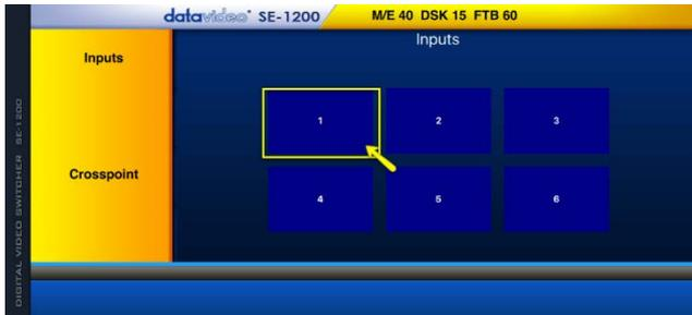
2. Six video input channel selection buttons will be displayed. **Click on the input channel button that you wish to Freeze.**
