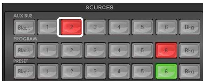
**Step 4:** Select the PiP image source on the **AUX BUS** row of the **SOURCES** panel. This will be shown over the chosen Preview image before being taken to Program/air with the next mix or wipe transition.
