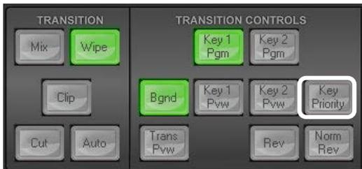
When Key 1 and Key 2 are both active in Preview (or Program), they may overlap each other on the screen. Using the Priority Button you can change the order of these keyers. The button acts in a toggle on/off way, i.e. Key1 over Key2 or Key2 over Key1.
