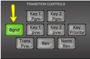
In order to wipe between two video sources first ensure the Background Transition or **Bgnd** button is ON / backlit green in the **transition controls** area of the user interface.
