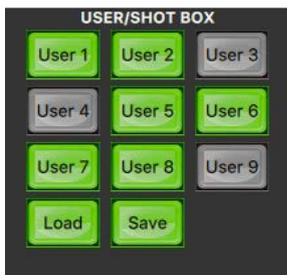
To load a previously saved SE-1200 MU Setup, simply click the **LOAD** button on the **USER/SHOT BOX** panel and an on-screen number pad will open.
