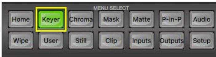
**Step 5:** To adjust the Luma key settings. Click the **Keyer button** in the **MENU SELECT panel** and the menu screen will appear as shown on the left here.
