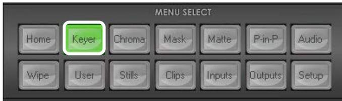
**Step 5:** To adjust the Luma key settings. Click the **Keyer button** in the **MENU SELECT** panel and the menu screen will appear as shown on the left here.
