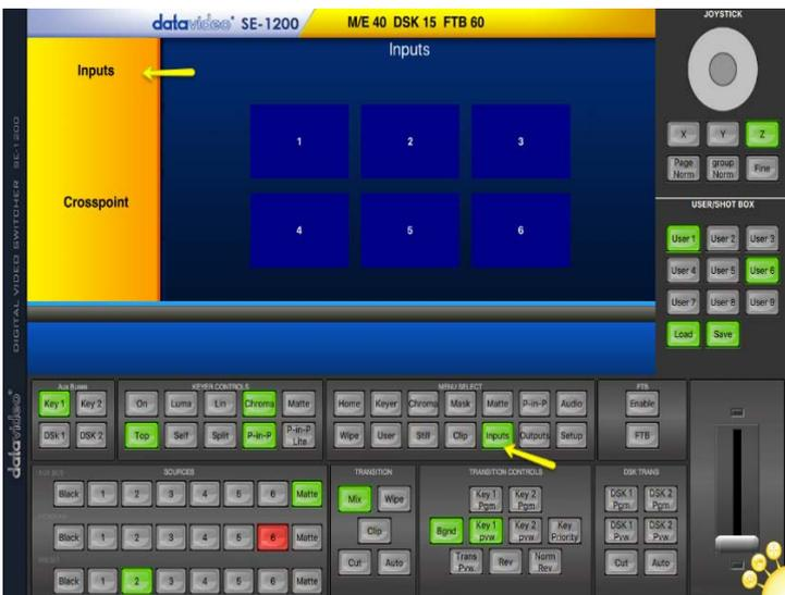
The physical input sources can be swapped around within the SE-1200 MU by using the **cross point** section of the **Inputs** menu.
