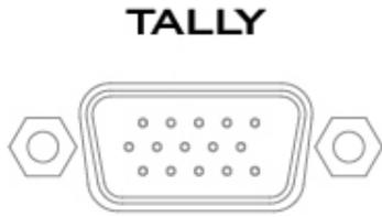
The SE-1200 MU has a D-sub 15 pin female tally output port. These connections provide bi-colour tally information to a number of other Datavideo products, such as the ITC-100 eight channel talkback system and the TLM range of LCD Monitors. The ports are open collector ports and as such do not provide power to tally light circuits.
