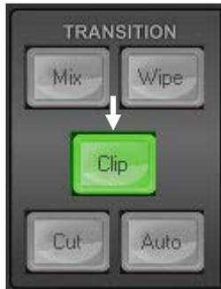
Clicking **Clip** will select the current wipe transition in use when moving from the current video source on the Program row to the selected next source on the Preset row.
