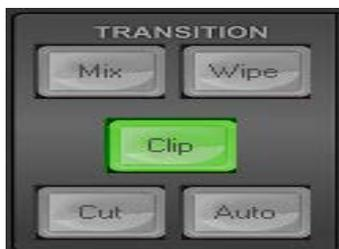
Clicking **Clip** will select the current wipe transition in use when moving from the current video source on the Program row to the selected next source on the Preset row.
