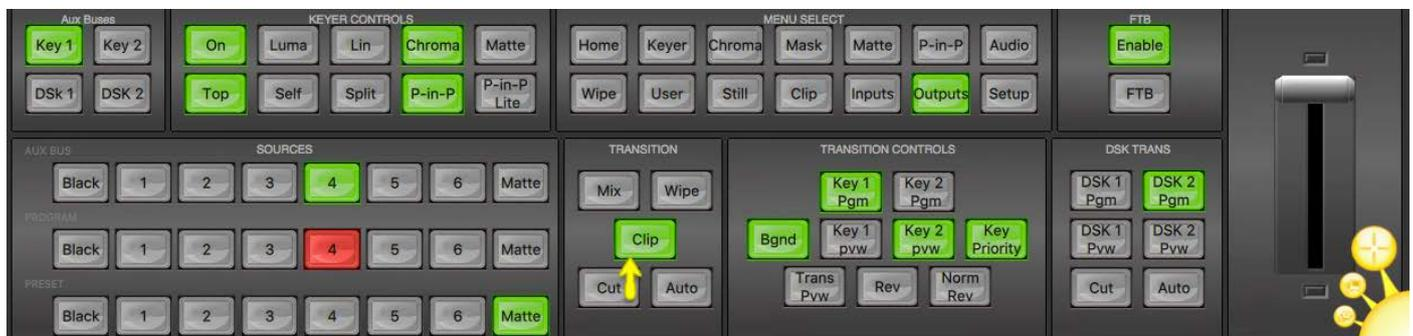
2. Selecting the next source on the lower **Preset row** of buttons and then pressing the **Cut** button.
