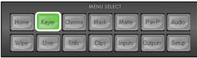
**Step 6:** To adjust the Luma key settings. Click the **Keyer button** in the **MENU SELECT** panel and the menu screen will appear as shown on the left here.
