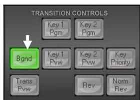
In order to wipe between two video sources first ensure the Background Transition or **Bgnd** button is ON / backlit green in the **transition controls** area of the user interface.
