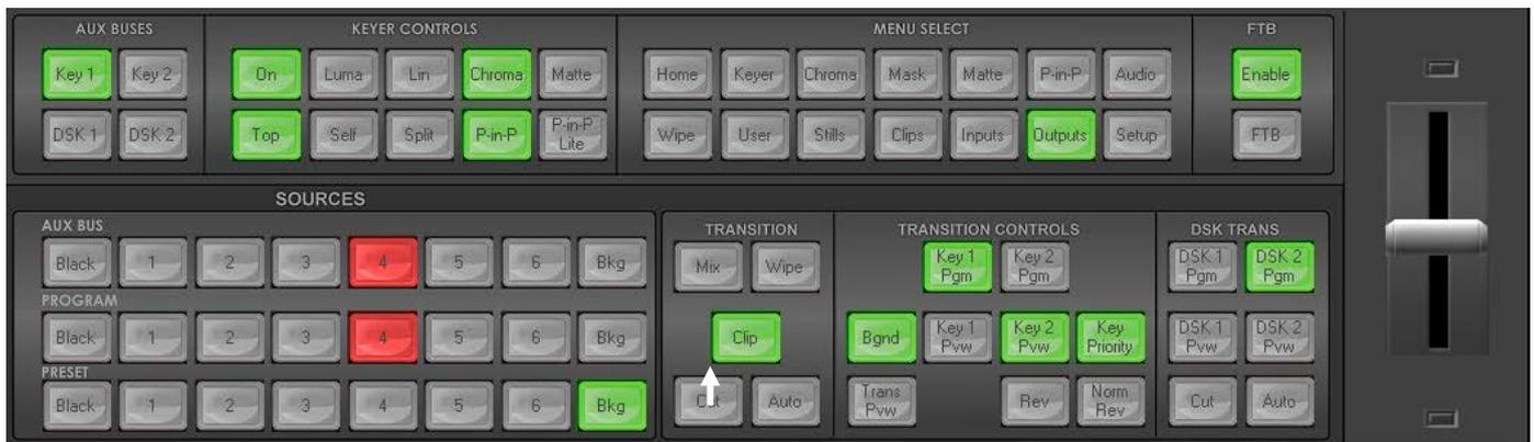
2. Selecting the next source on the lower **Preset row** of buttons and then pressing the **Cut** button.
