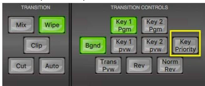
Using the Priority Button you can change the order of these keyers. The button acts in a toggle on/off way, i.e. Key1 over Key2 or Key2 over Key1.
