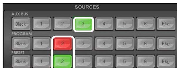
**Step 3:** The **Split button** is **backlit green**, select the CG **key source** on the **AUX BUS Row** (input 3).
