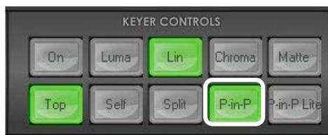
**Step 2:** Select the Key 2 effect by clicking the **P-in-P** button (backlit green) in the **Keyer Controls** panel.
