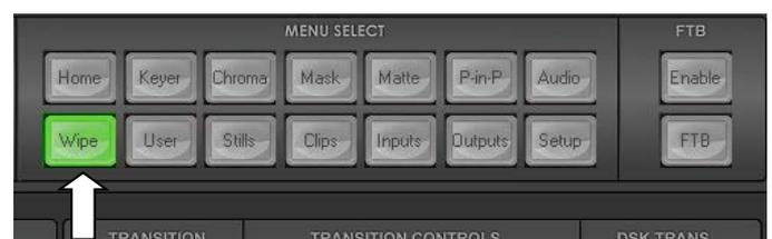
Each wipe pattern consists of blue and white colours. The white represents the current Program image (A) and the blue represents the WIPE-IN image (B). There are a total of 32 WIPE presets offered by the SE-1200 MU as shown below.
