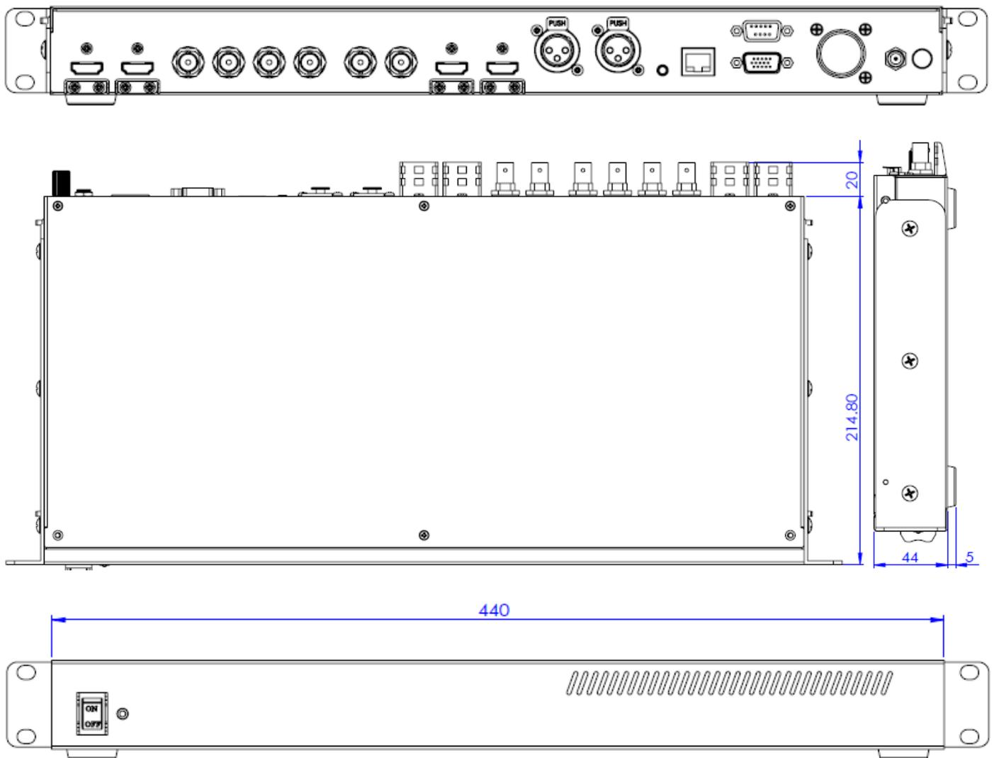
All measurements in millimetres (mm)
