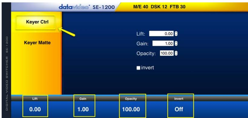
The options in the blue bar along the bottom of the Screen will allow you to calibrate for a white or black key using the **Lift, Gain, Opacity** and **Invert Functions**. The [Keyer Control section \(7.1.1\)](#) will explain the effects of **Lift, Gain, Opacity** and **Invert**.
