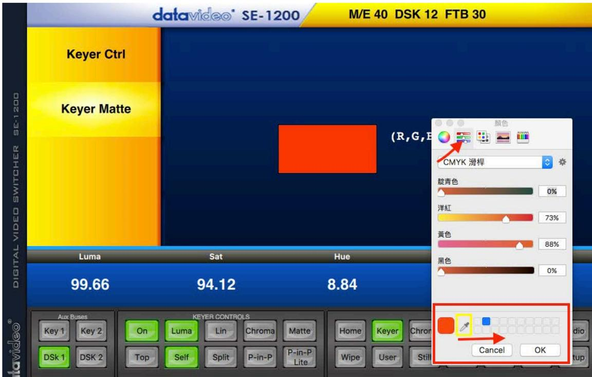
1. Select the second option which is the **color selection ruler** as the arrow pointed. And then click the drop-down menu to select different color selection tool such as the **Gray Scale color slider**, **RGB color slider**, **CMYK color slider** and **HSB color slider**.
