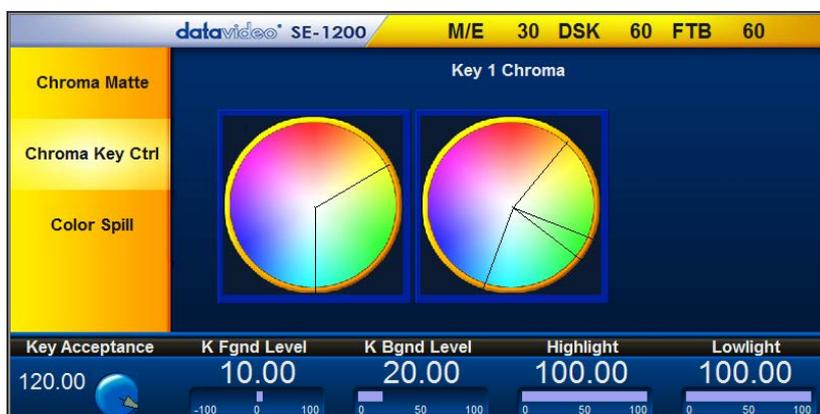
The **Chroma Key Ctrl** parameters and values are shown along the bottom of the display. Two colour palettes, **Main** and **Chroma**, are shown in the diagram.
