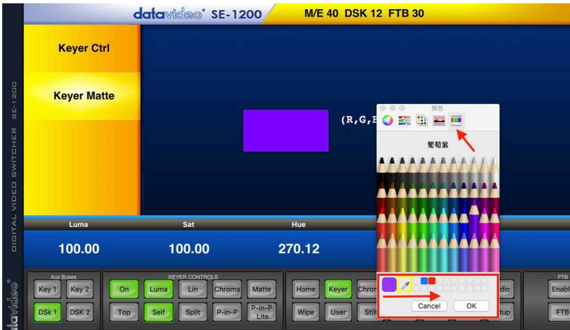
1. Select the fifth option which is the **Pencil** as the arrow pointed and then users can select needed color from different color pencils as shown in the picture.
