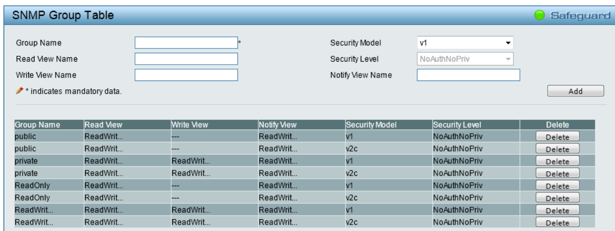
Figure 4.113 – SNMP > SNMP > SNMP Group
