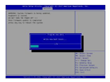
5. After the BIOS recovery process is completed, press any key to reboot the system.
